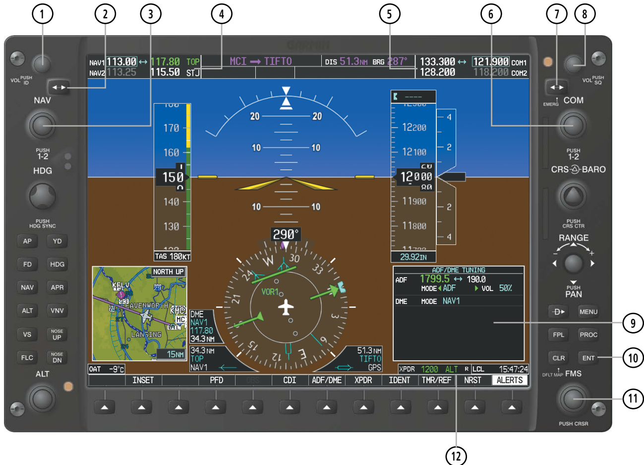
Figure 4-1 MFD/PFD Controls, NAV/COM Frequency Tuning Boxes, and ADF/DME Tuning Window (PFD Shown)
