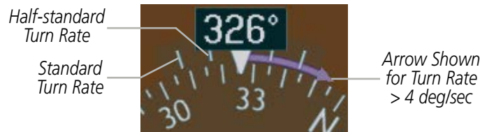
Figure 2-19 Turn Rate Indicator and Trend Vector
