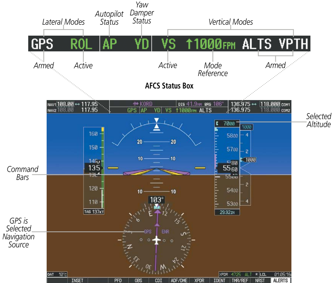
Figure 7-2 PFD AFCS Display
