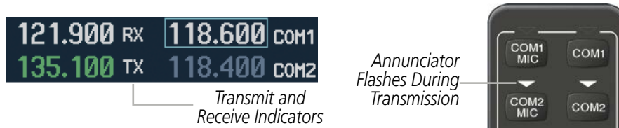
Figure 4-4 COM Radio Transmit and Receive Indications
