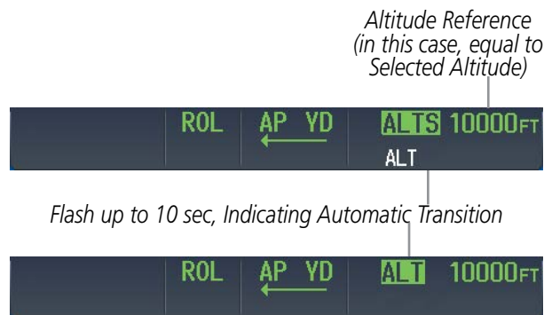
Figure 7-7 Automatic Mode Transitions During Altitude Capture
