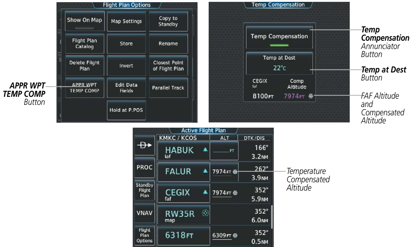
Figure 5-173 Temperature Compensation for Approach Waypoints
