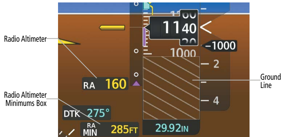
Figure 2-57 Altimeter Displaying the Ground Line (RAD ALT)
