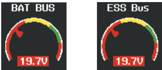
Battery and Essential Bus Low Voltage
