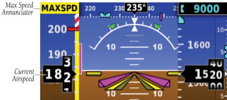
Figure 4-1 ESP Engaged - High Airspeed
