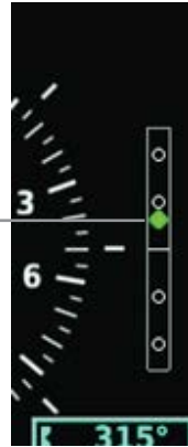
Figure 2-28 Vertical Deviation Indicator (Glideslope-ILS Source) - HSI
