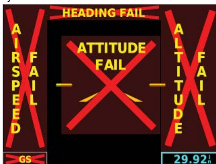
Figure 1-2 G5 Failure Annunciations
