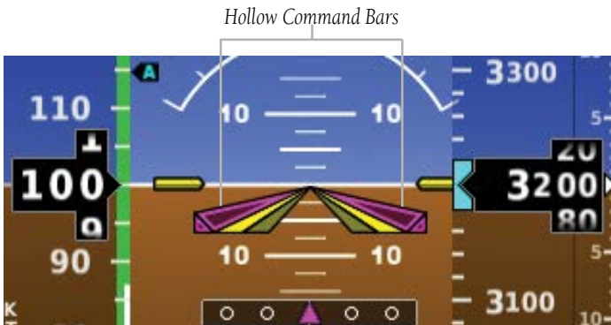
Figure 3-5 Command Bars - Hollow (Pilot Hand Flying)
