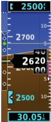
Figure 2-27 Vertical Deviation Indicator (Glideslope-ILS Source) - PFD
