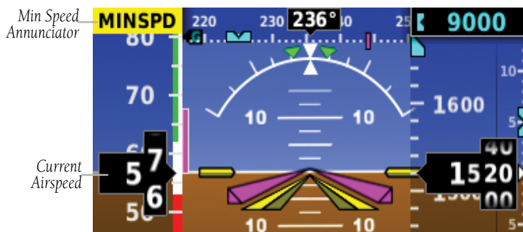
Figure 4-2 ESP Engaged - Low Airspeed
