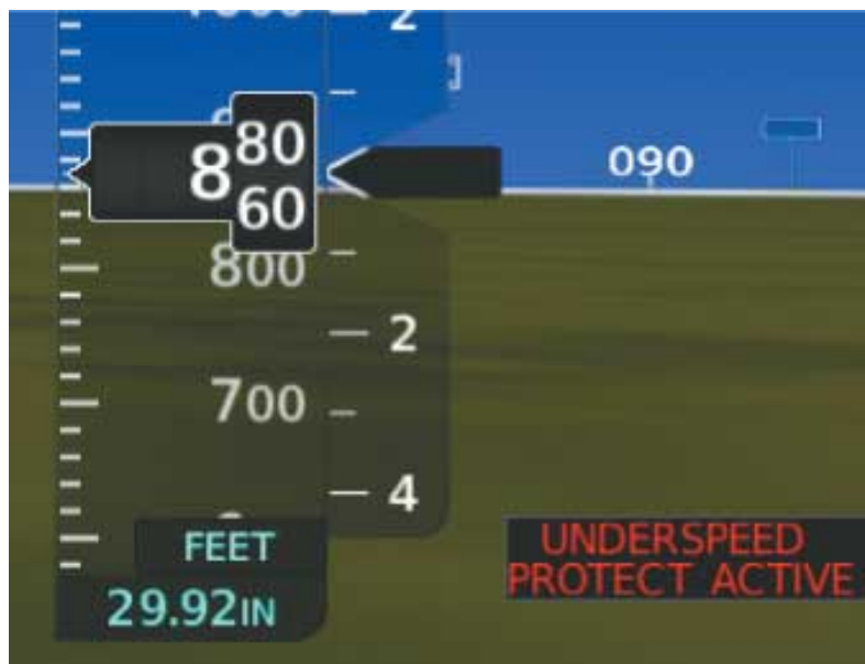
Figure 7-31 Underspeed Protect Active Annunciation
