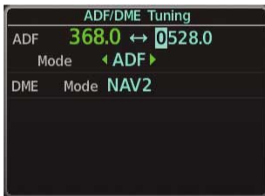
Figure 4-14 Entering ADF Standby Frequencies
