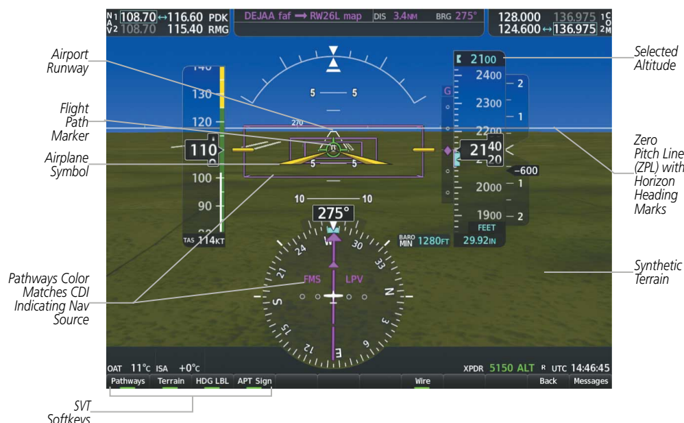
Figure 2-38 SVT on the Primary Flight Display
