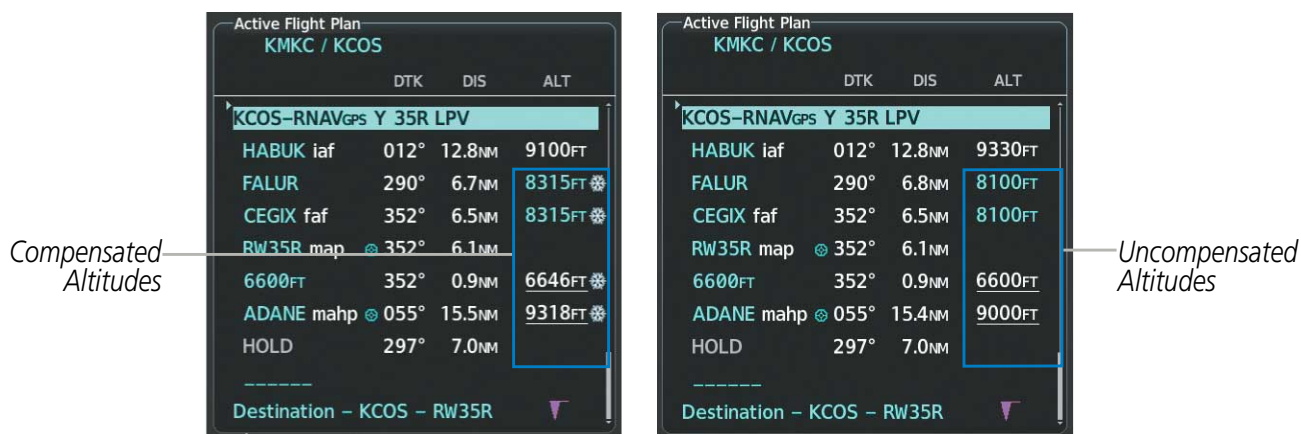
Figure 5-84 Temperature Compensation in the Active Flight Plan
