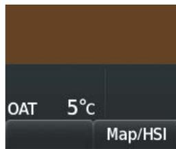
Figure 2-28 Outside Air Temperature
