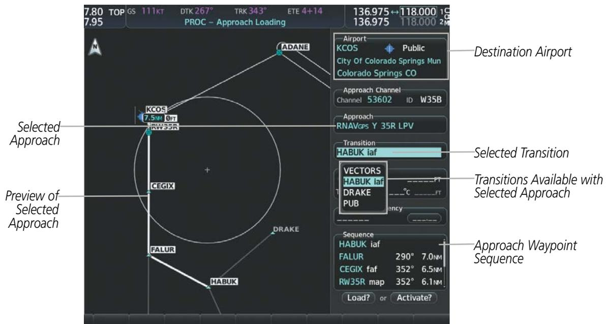
Figure 5-61 Approach Loading Page - Selecting the Transition
