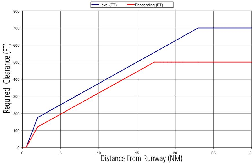
Figure 6-60 FLTA Alert Minimum Terrain and Obstacle Clearance Values
