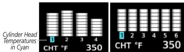
Figure 3-12 Cylinder Head Temperatures (CHT)
