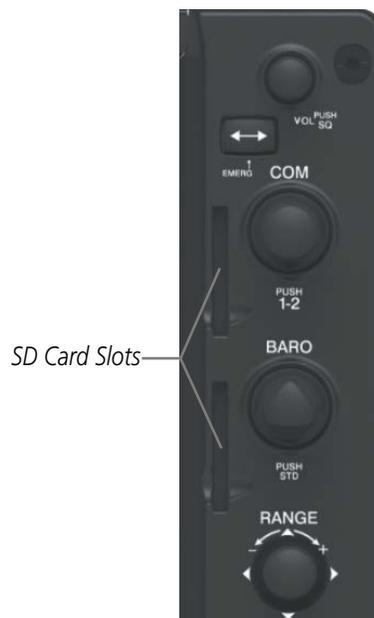
Figure 1-3 PFD/MFD Display Bezel SD Card Slots
