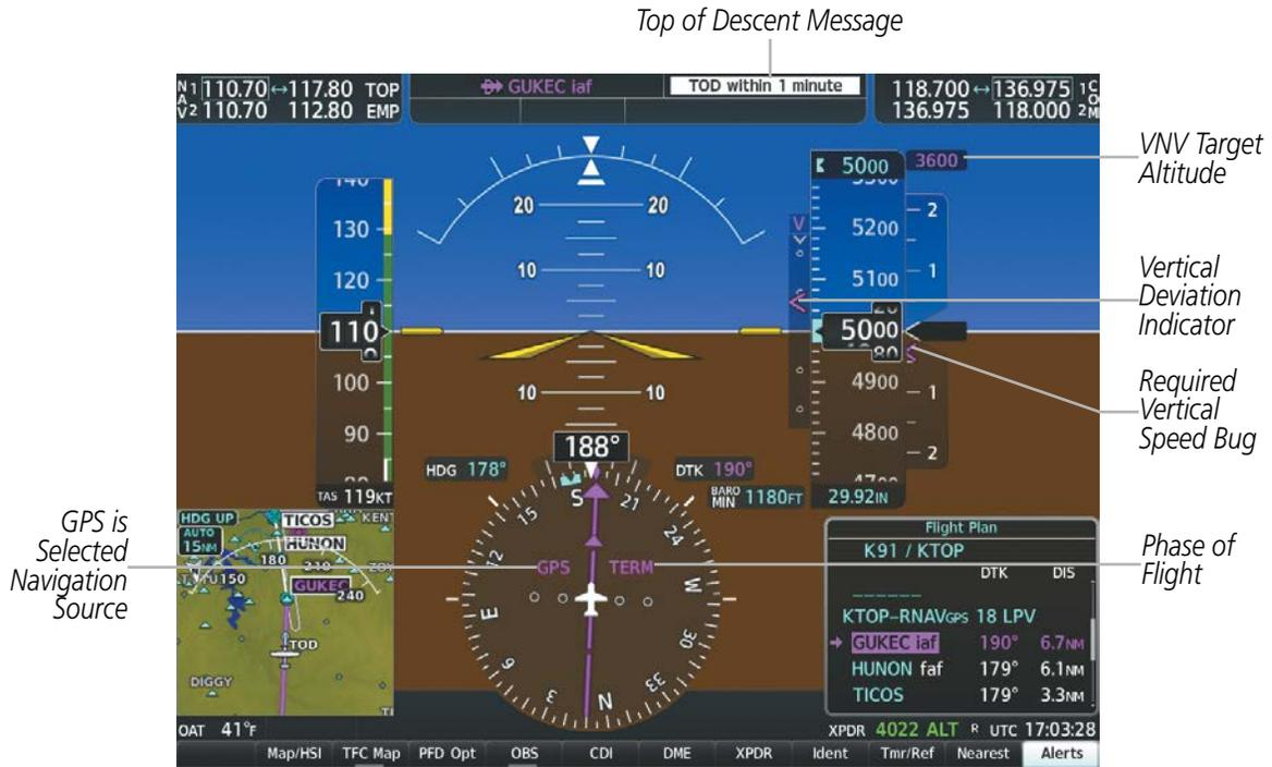
Figure 2-30 Vertical Navigation Indications (PFD)
