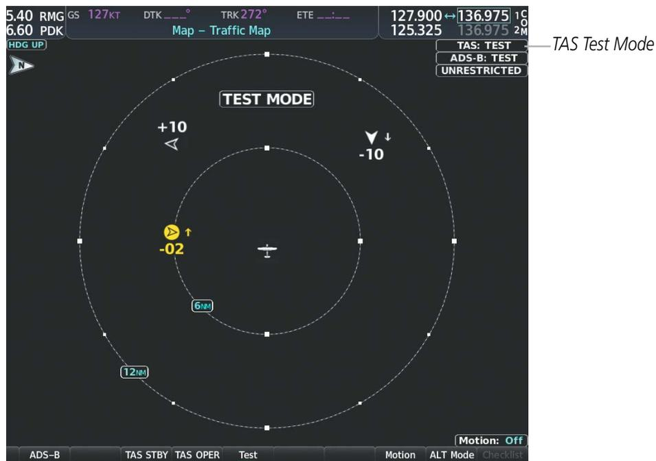
Figure 6-70 System Test in Progress with Test Pattern
