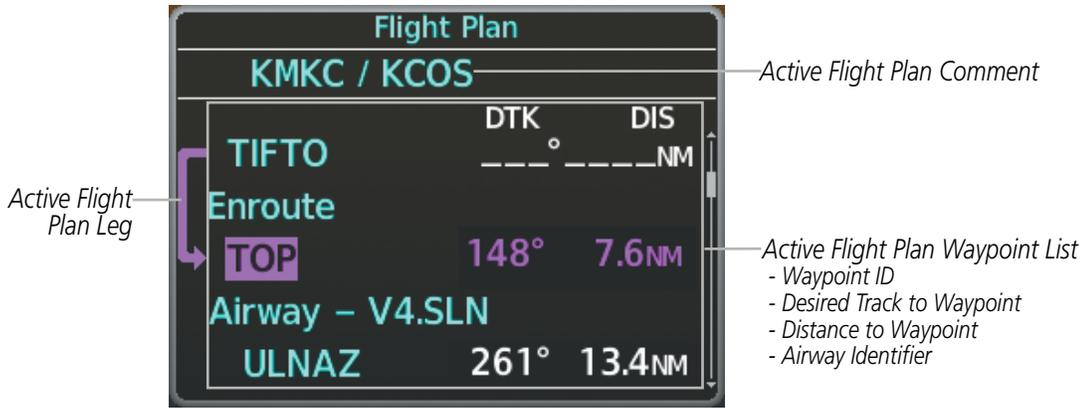
Figure 5-48 Active Flight Plan Window on PFD
