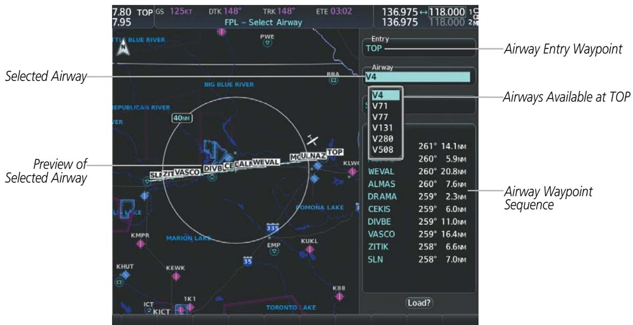
Figure 5-53 Select Airway Page - Selecting Airway
