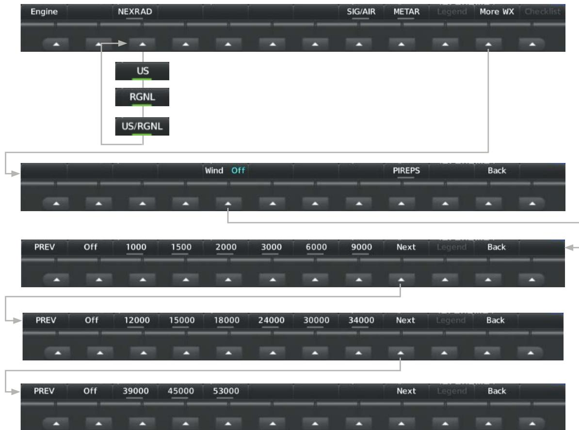
Figure 6-5 Weather Data Link (FIS-B) Weather Product Softkeys
