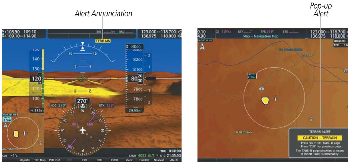
Figure 6-58 TAWS-B Alert Annunciations
