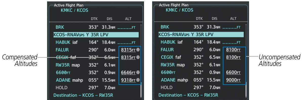
Figure 5-81 Temperature Compensation in the Active Flight Plan
