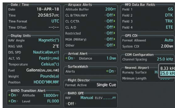
Figure 4-9 Frequency Channel Spacing
