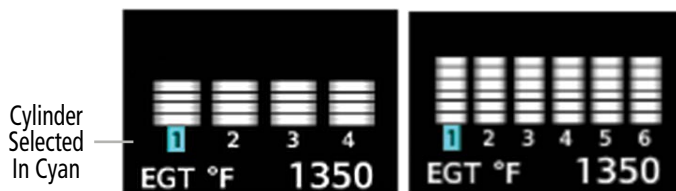
Figure 3-11 Exhaust Gas Temperatures (Normal)
