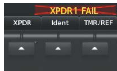
Figure 4-38 Transponder Fail Indication
