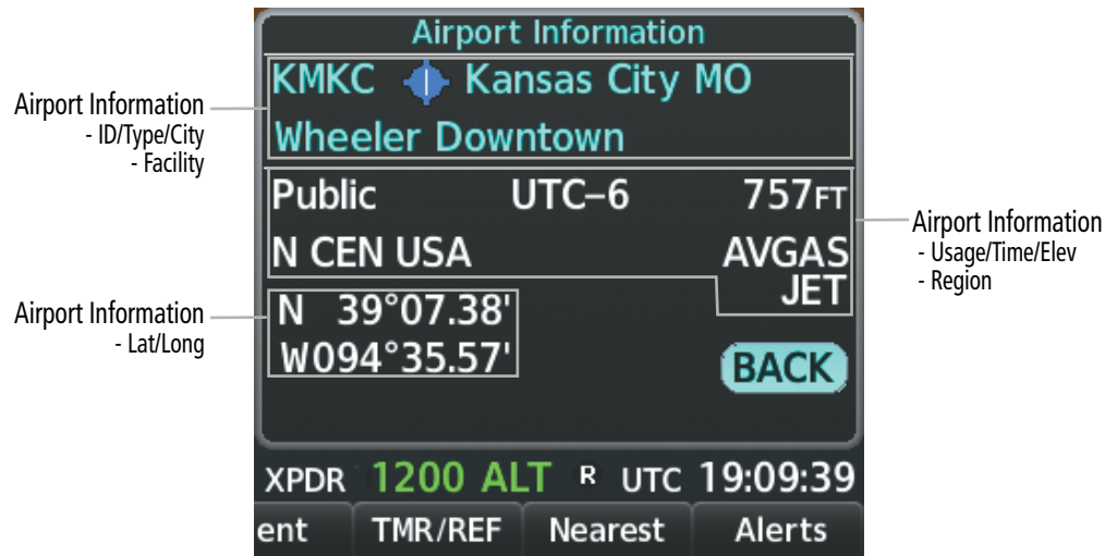
Figure 5-28 Airport Information on PFD
