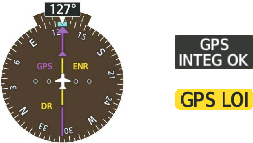
Figure 2-38 Example HSI Annunciations
