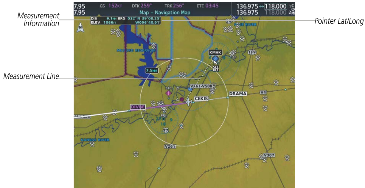
Figure 5-11 Navigation Map - Measuring Bearing and Distance
