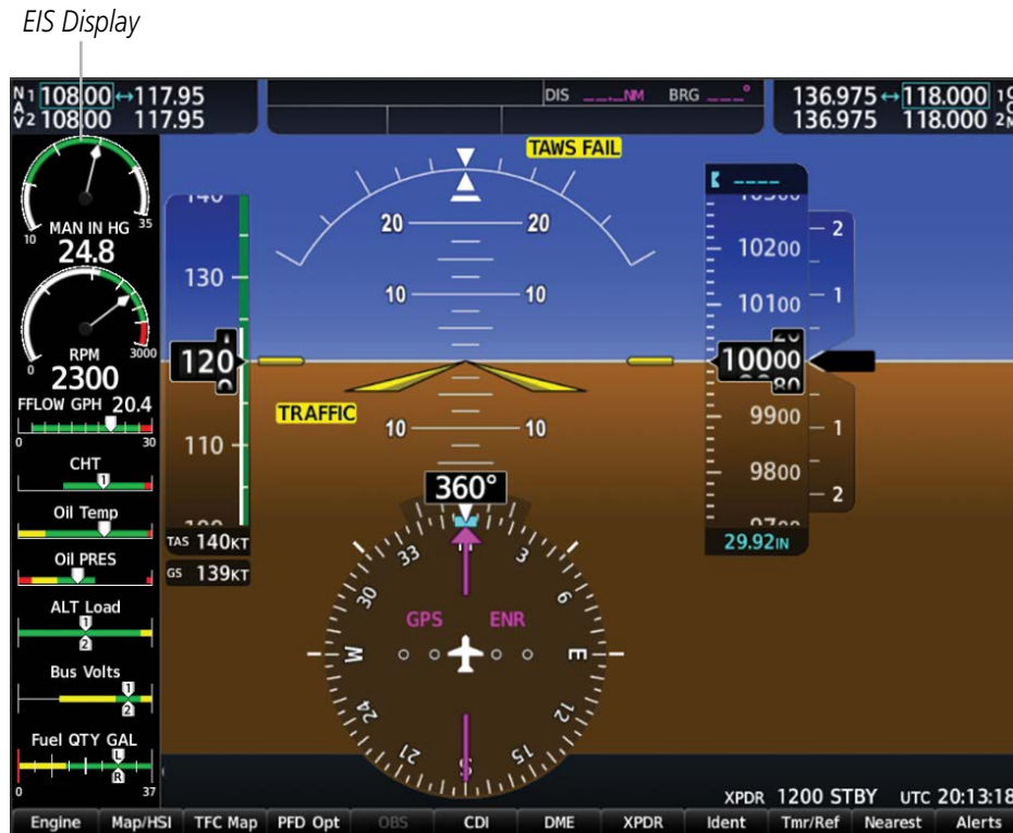
Figure 3-7 Reversionary Mode (EIS Shown)
