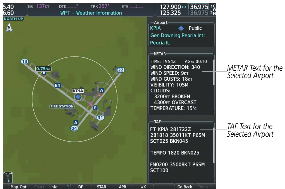
Figure 6-28 METAR and TAF Text on the Weather Information Page
