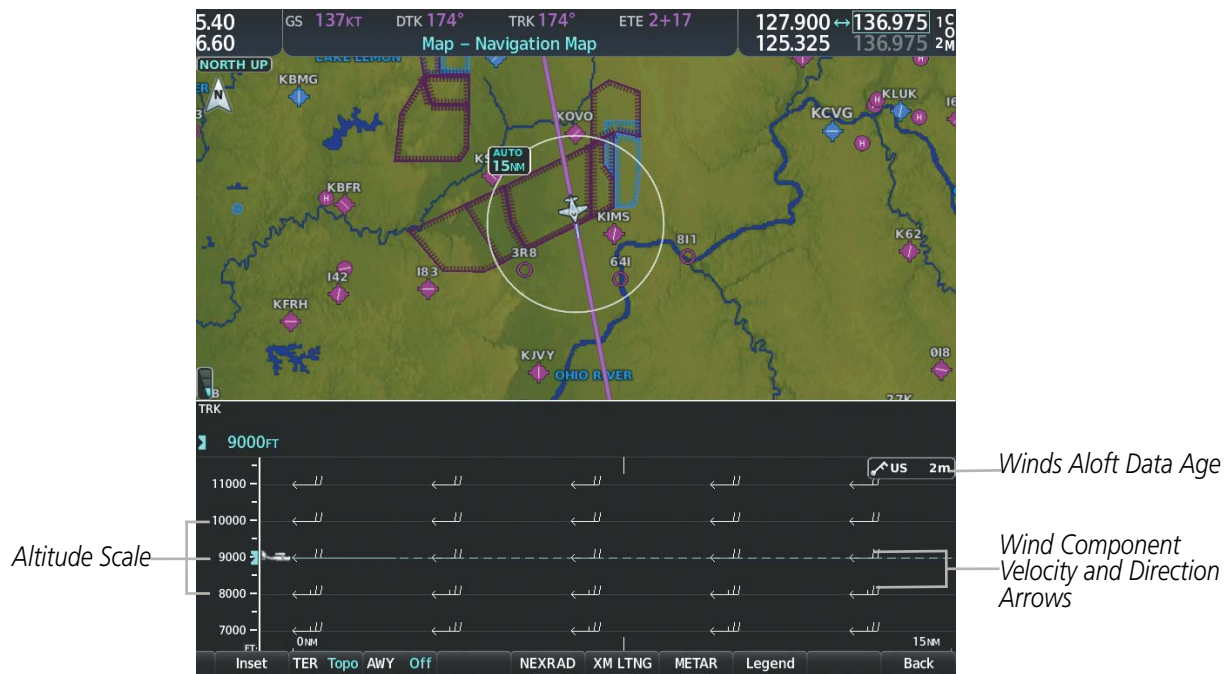
Figure 6-36 Navigation Map Page with Winds Aloft Data on Profile View
