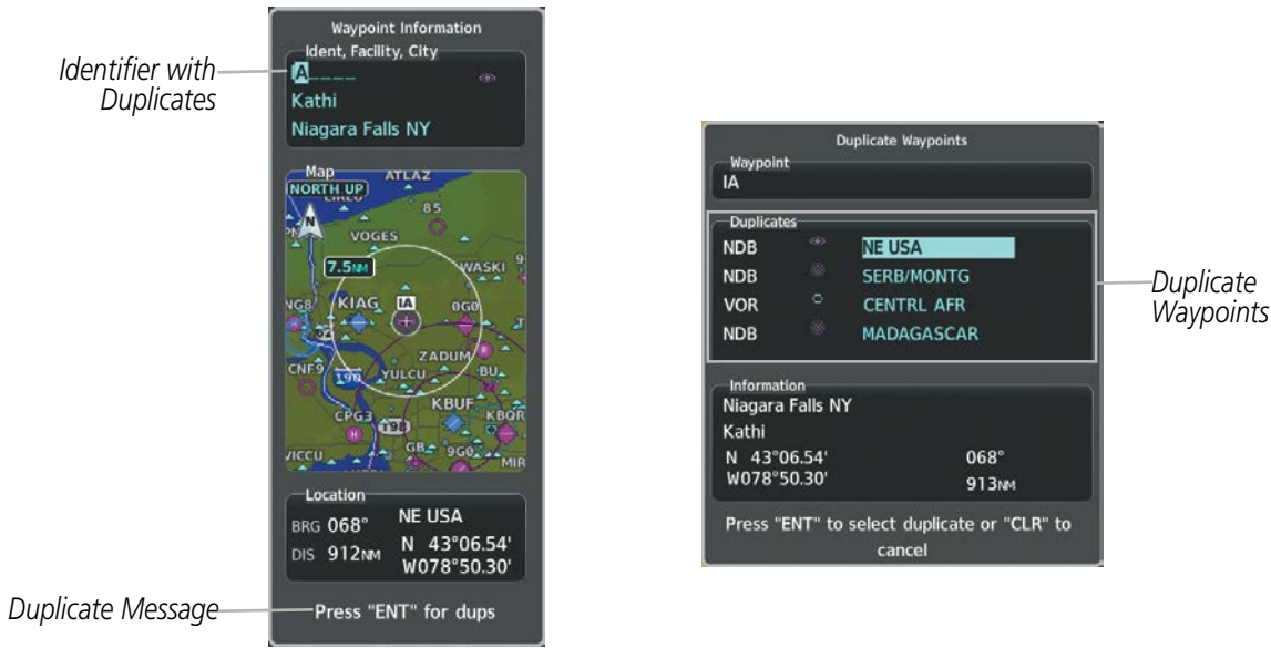
Figure 5-25 Waypoint Information Window - Duplicate Identifier
