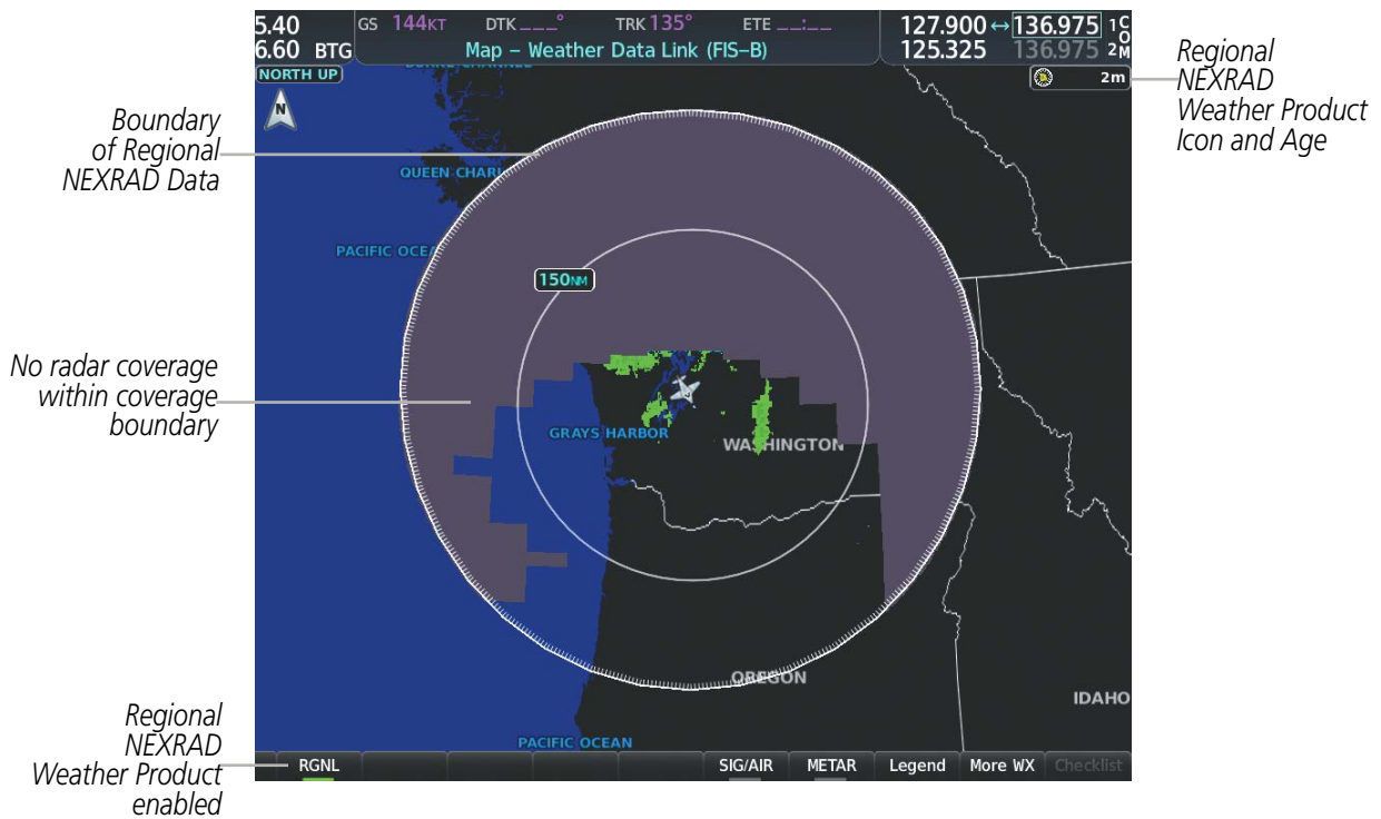
Figure 6-11 Regional NEXRAD Weather Product on the Weather Data Link (FIS-B) Page
