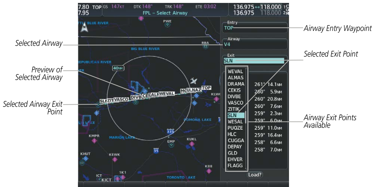
Figure 5-54 Select Airway Page - Selecting Exit Point
