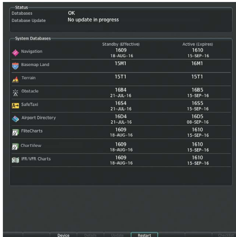
Figure B-11 Database Page with Updated Databases
