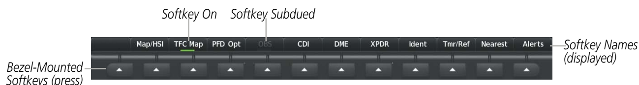
Figure 1-9 Softkeys (First-Level PFD Configuration)
