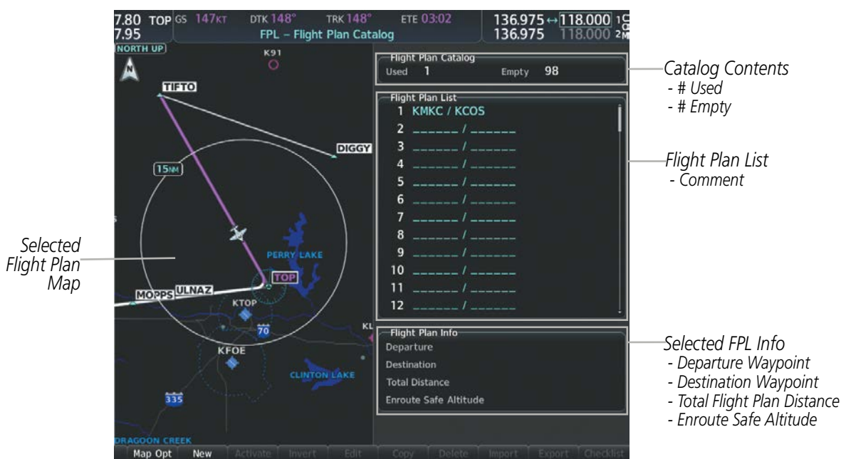
Figure 5-49 Flight Plan Catalog Page
