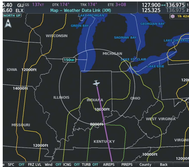
Figure 6-32 Freezing Level Data
