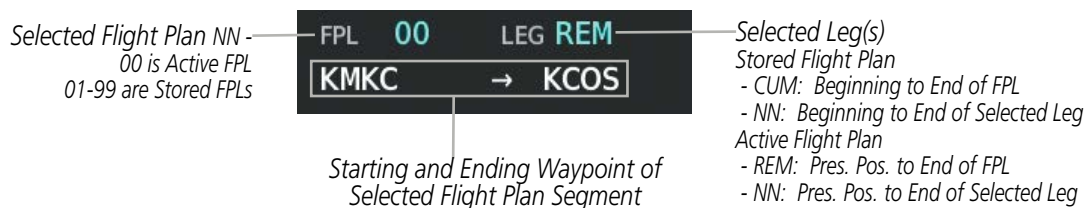
Figure 5-83 Trip Planning Page - Flight Plan Mode
