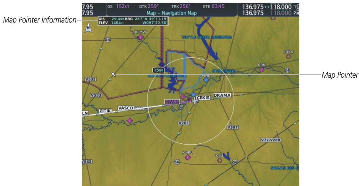
Figure 5-9 Navigation Map - Map Pointer Activated
