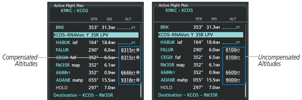
Figure 5-81 Temperature Compensation in the Active Flight Plan
