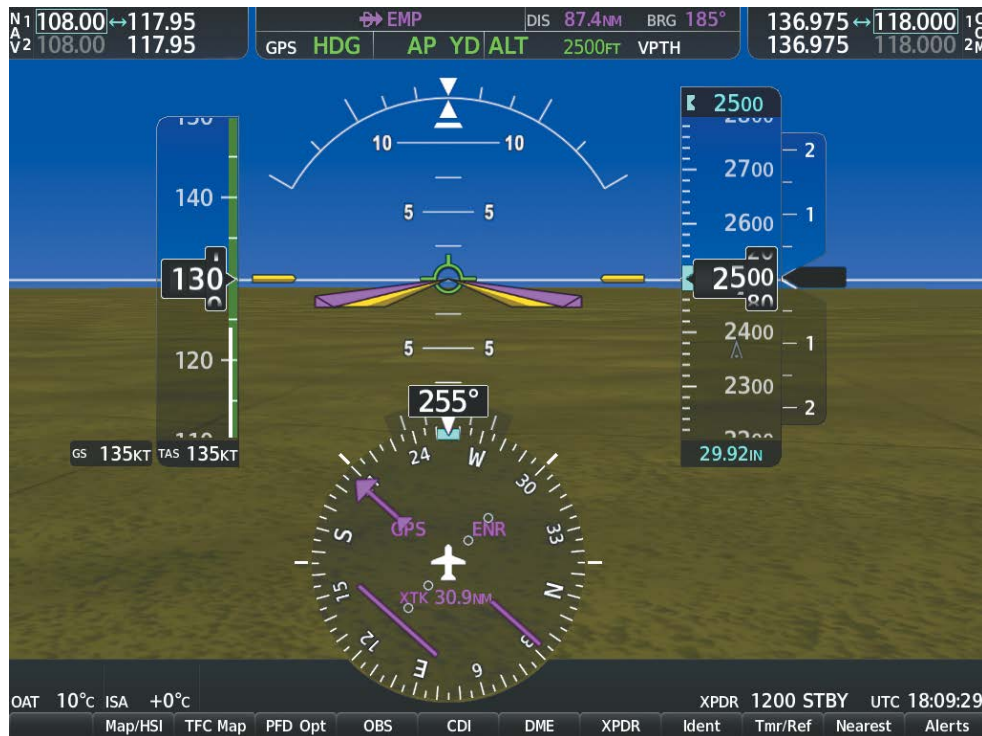
Figure 8-1 Synthetic Vision Imagery
