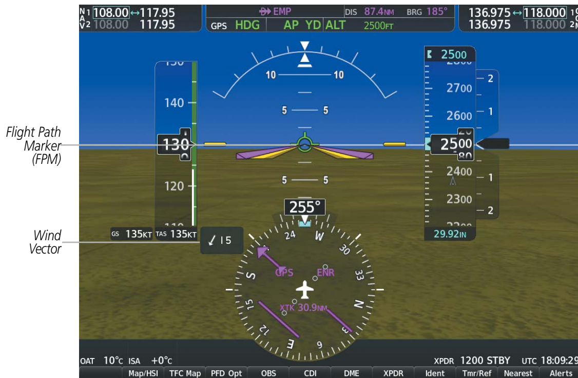
Figure 8-6 Flight Path Marker and Pathways
