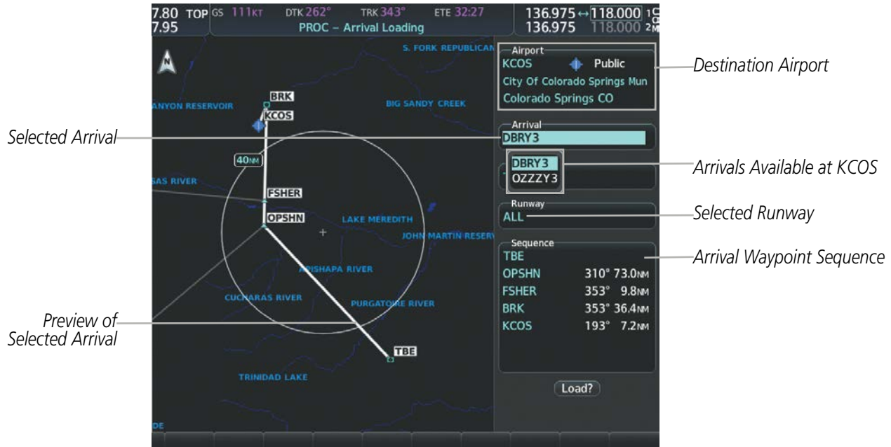
Figure 5-58 Arrival Loading Page - Selecting the Arrival
