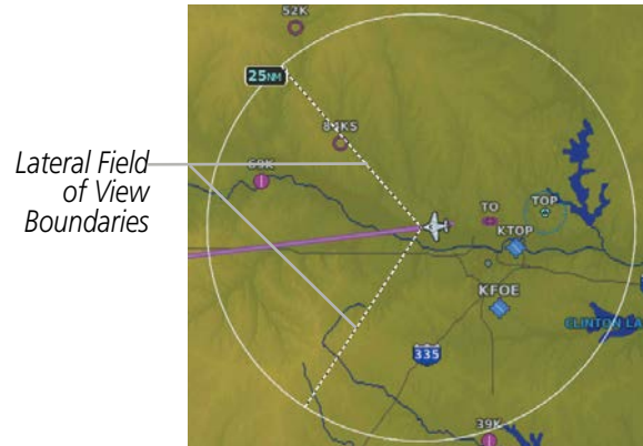
Figure 5-19 Navigation Map - Field of View
