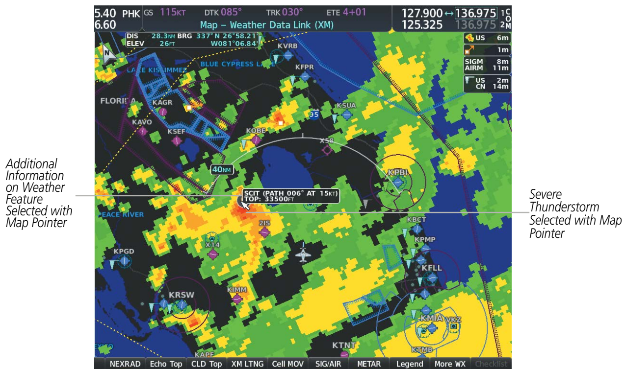
Figure 6-6 Panning on the Weather Data Link (XM) Page
