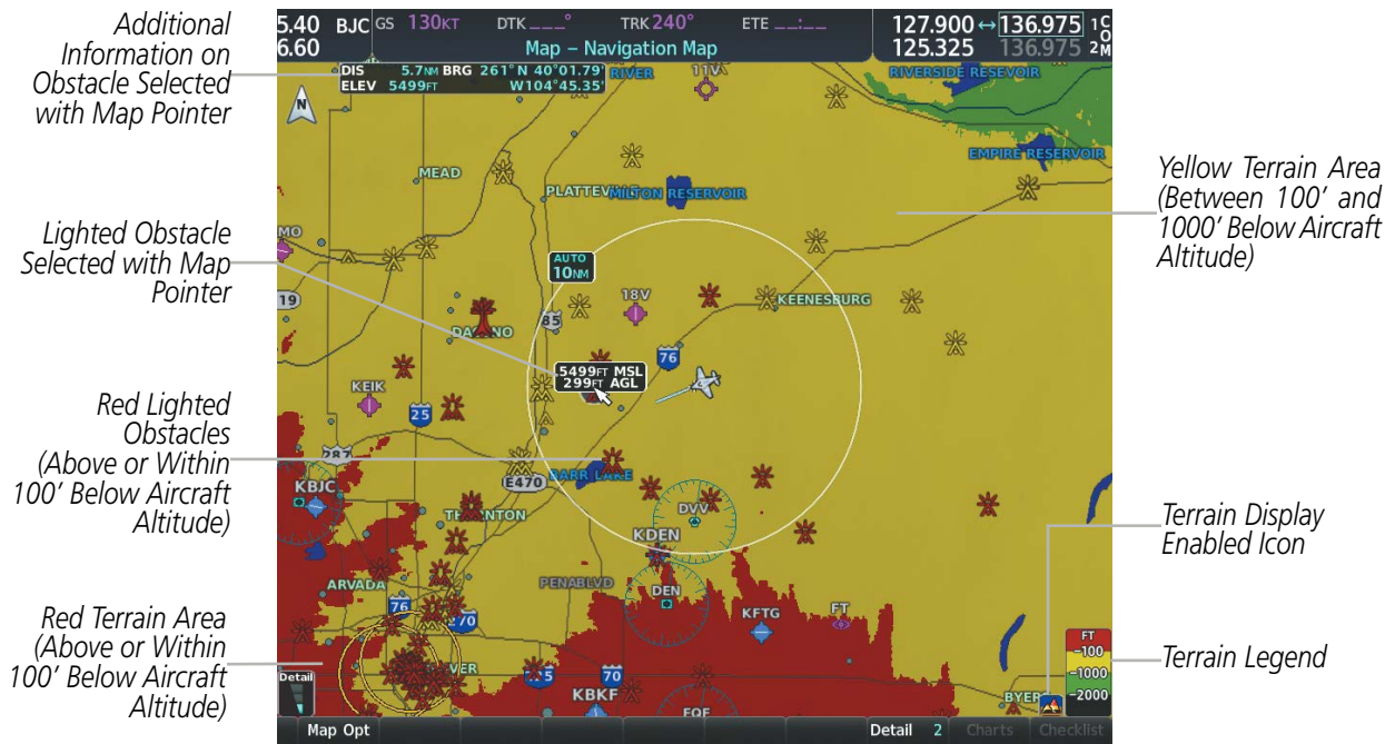
Figure 6-55 Terrain Information on the Navigation Map Page
