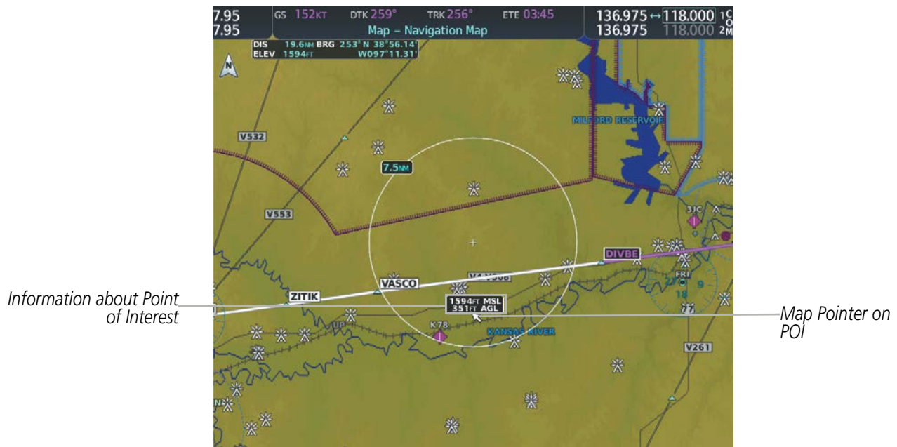
Figure 5-10 Navigation Map - Map Pointer on Point of Interest
