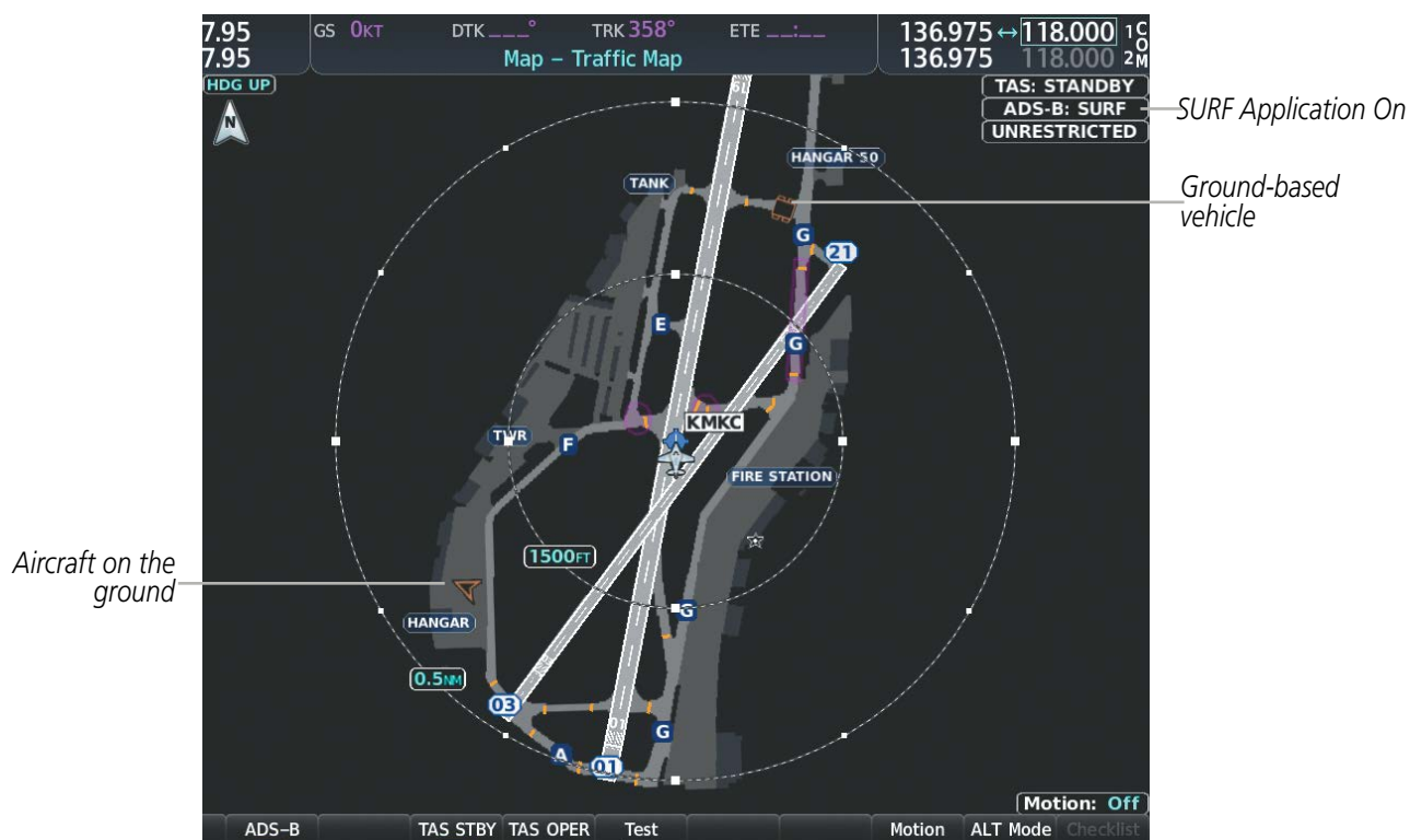
Figure 6-75 Traffic Map Page with SURF Mode On
