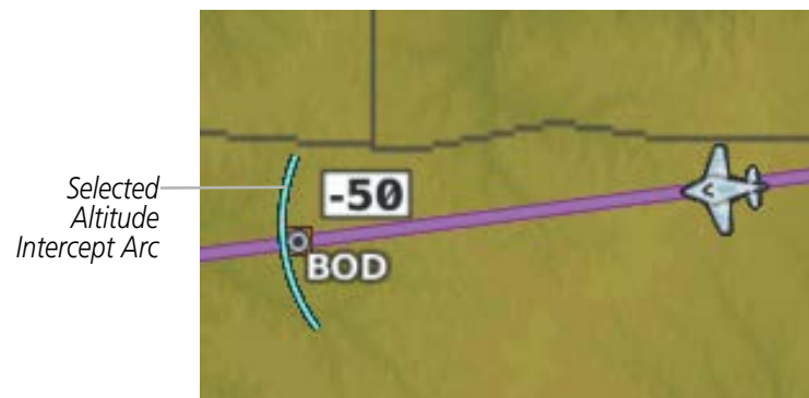
Figure 5-20 Navigation Map - Range to Altitude Arc
