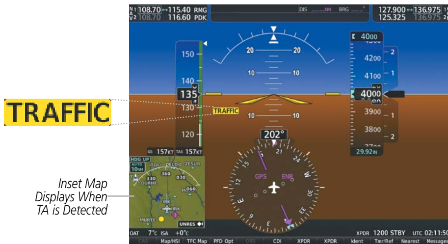
Figure 6-66 Traffic Annunciation (PFD)
