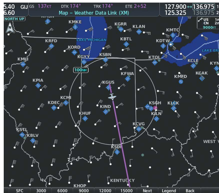
Figure 6-34 Winds Aloft Data at 12,000 Feet
