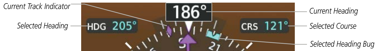
Figure 2-17 Heading and Course Indications
