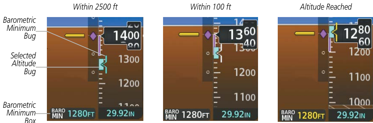
Figure 2-36 Barometric MDA/DH Alerting Visual Annunciations
