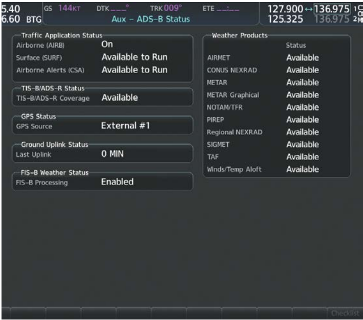
Figure 6-80 Viewing ADS-B Traffic Status on ADS-B Status Page
