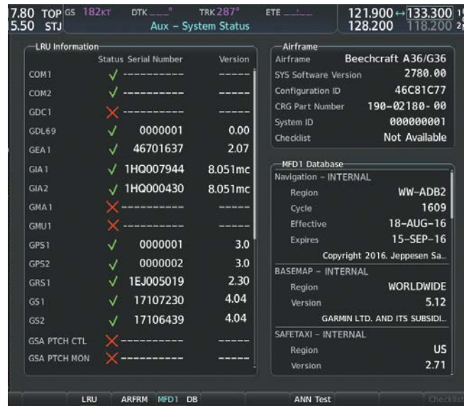
Figure 1-6 Example System Status Page
