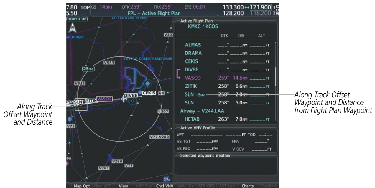
Figure 5-63 Along Track Offset
