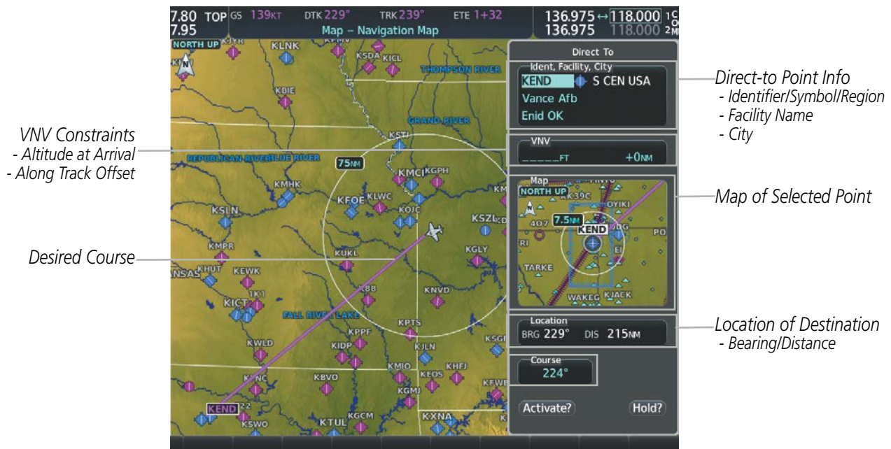
Figure 5-44 Direct-to Window - MFD
