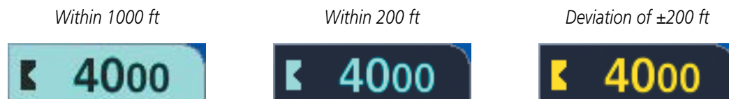
Figure 2-34 Altitude Alerting Visual Annunciations
