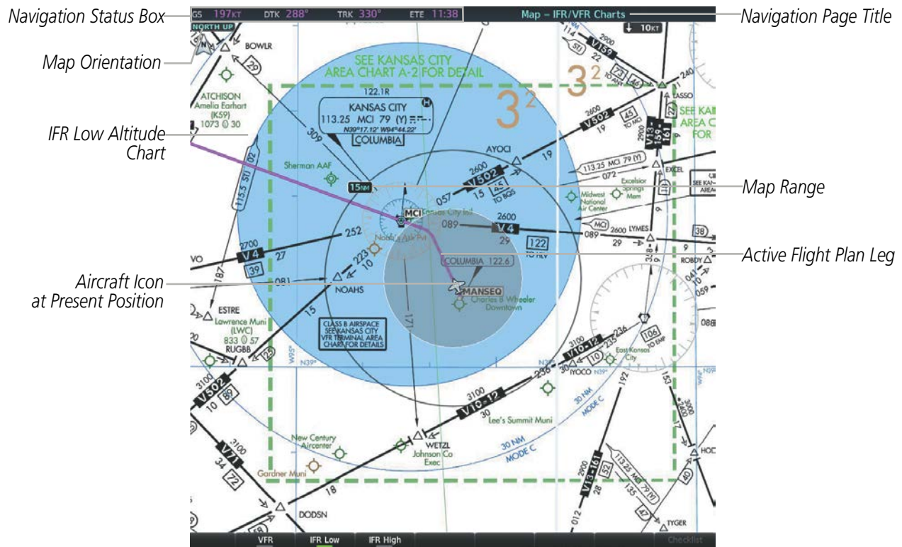
Figure 5-22 GPS Navigation Information on the IFR Low Altitude Chart
