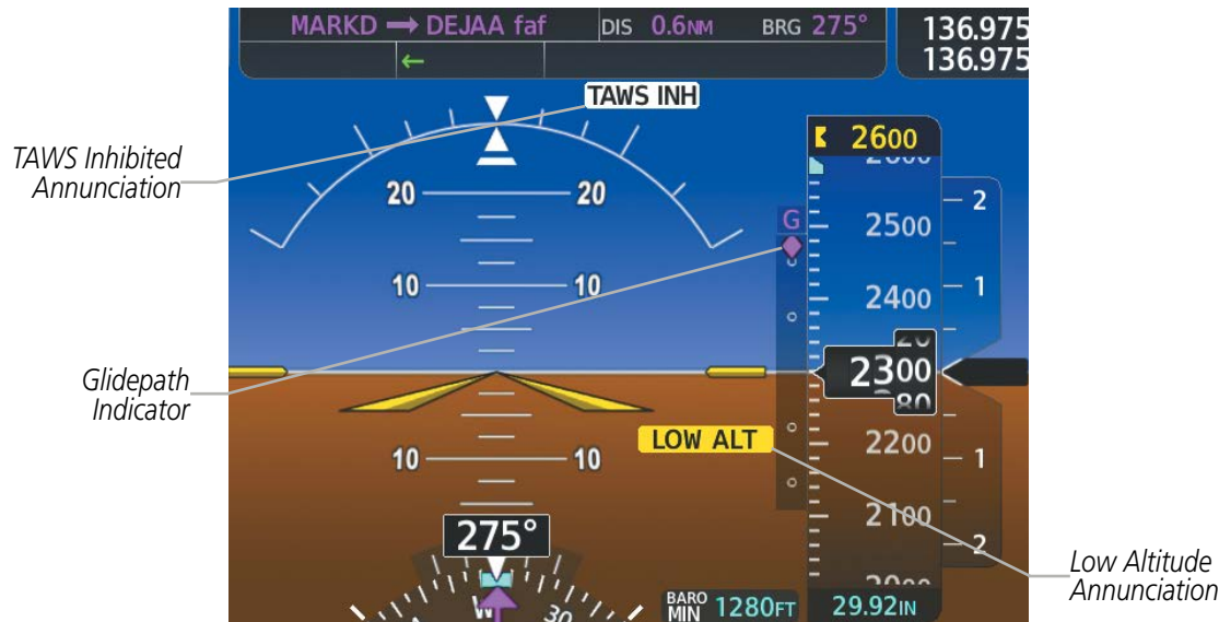
Figure 2-35 Low Altitude on GPS SBAS Approach
