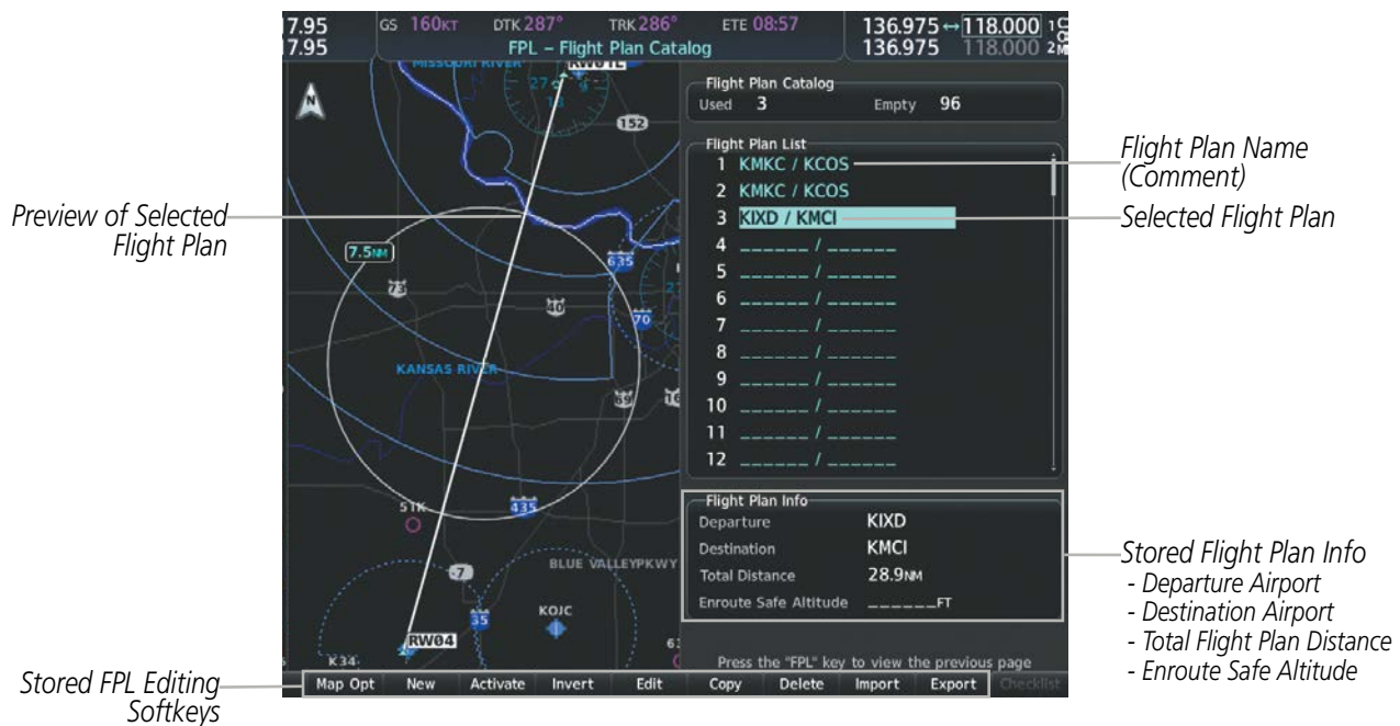
Figure 5-62 Stored Flight Plan Information
