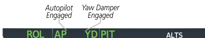
Figure 7-26 Autopilot and Yaw Damper Engaged
