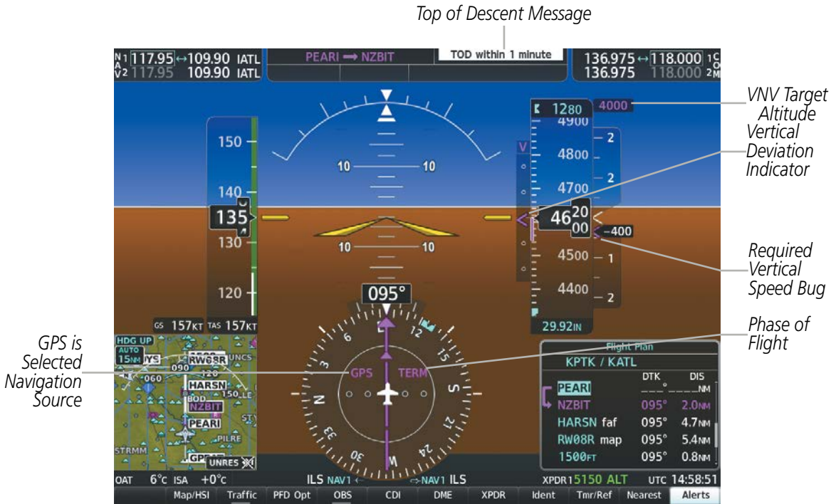
Figure 2-32 Vertical Navigation Indications (PFD)
