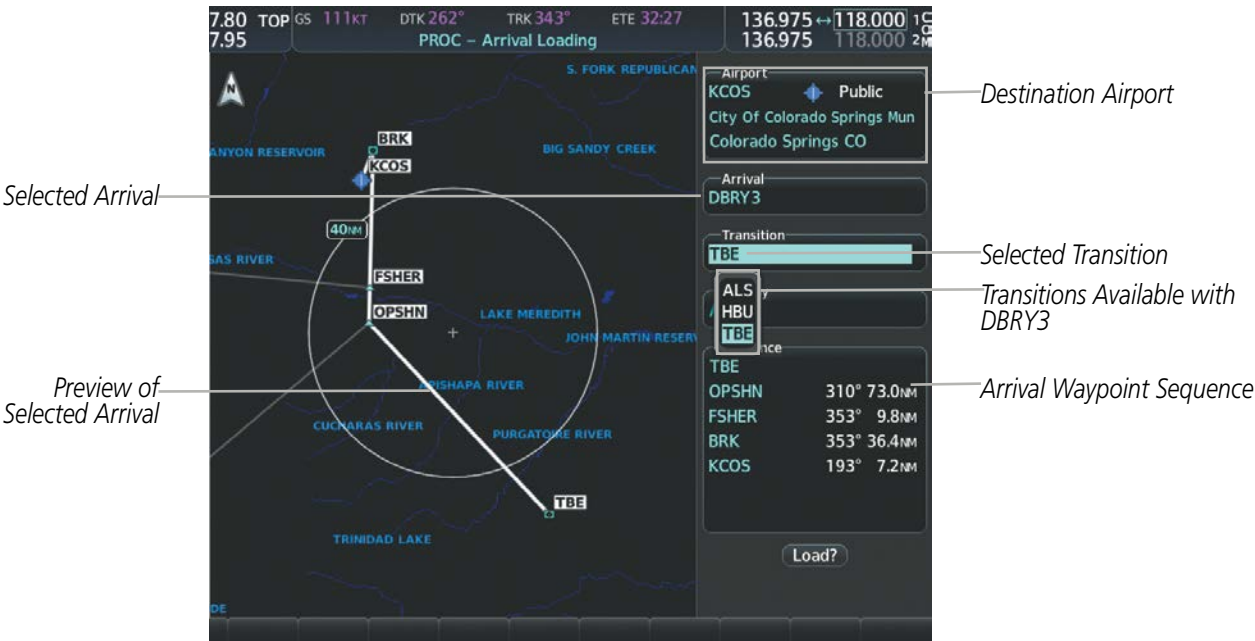
Figure 5-59 Arrival Loading Page - Selecting the Transition
