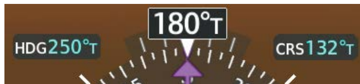
Figure 2-18 Heading and Course Indications (True)
