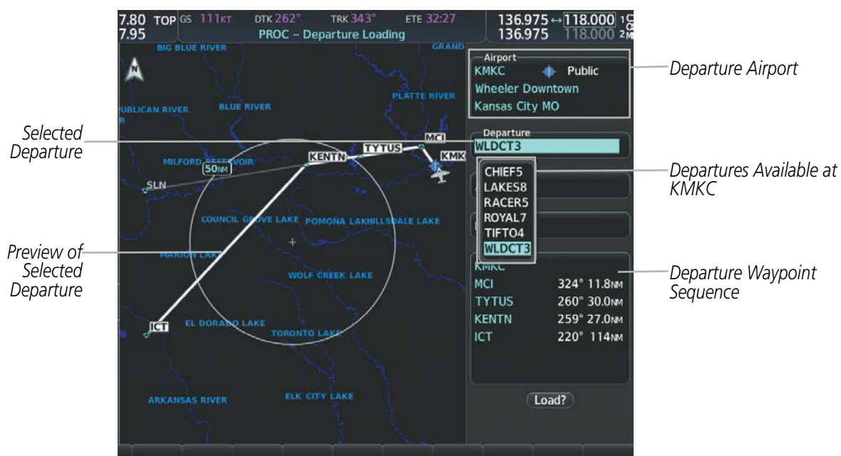
Figure 5-56 Departure Loading Page - Selecting the Departure
