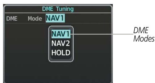
Figure 4-13 DME Tuning Window
