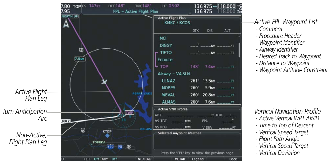
Figure 5-47 Active Flight Plan Page
