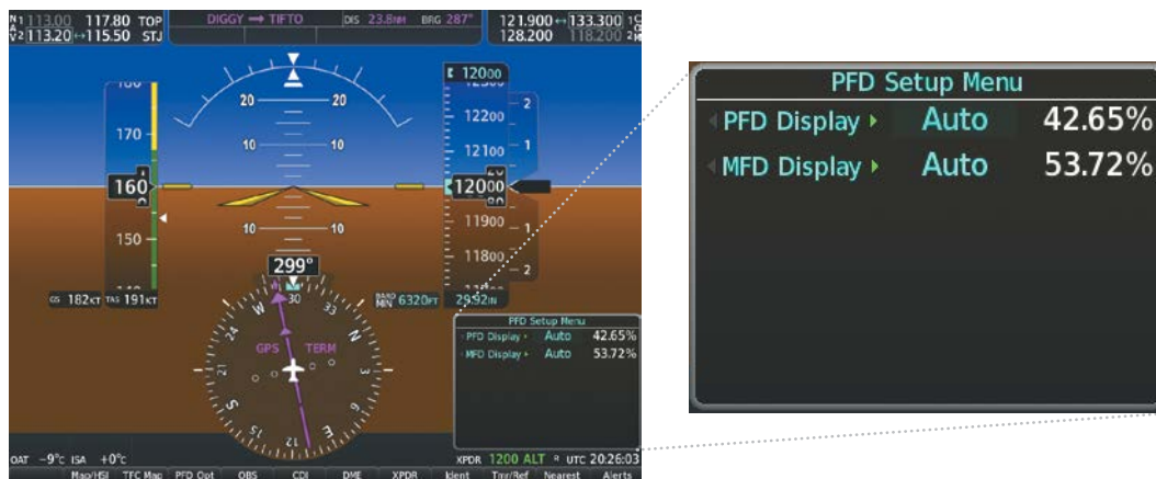
Figure 1-20 PFD Setup Menu
