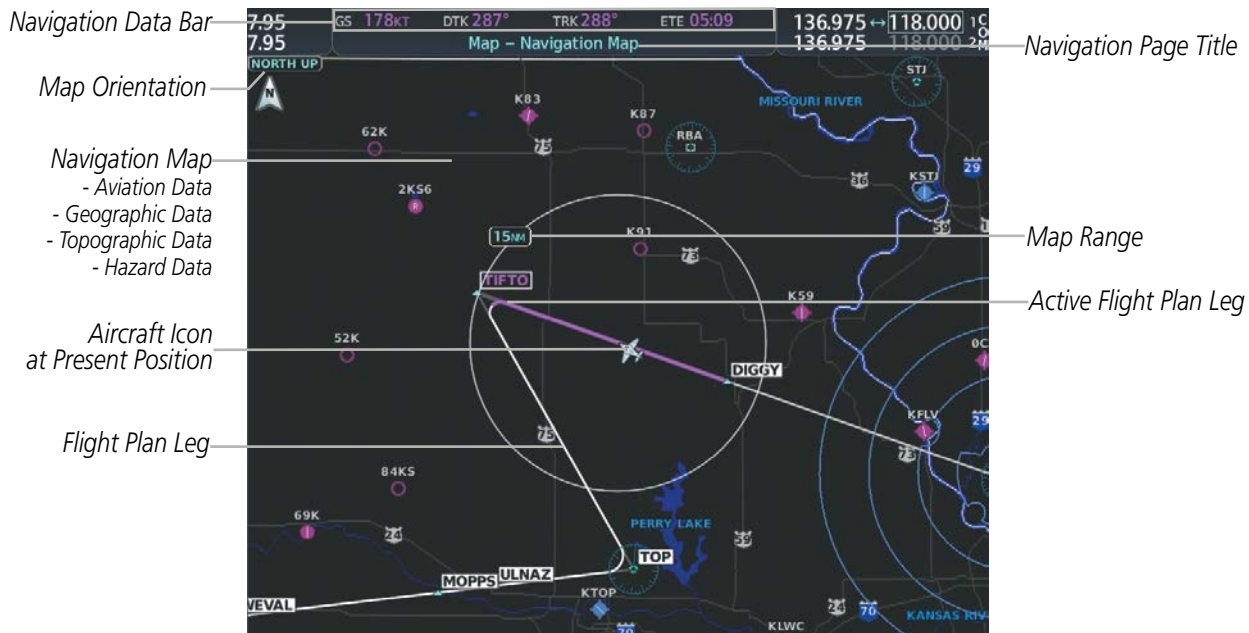
Figure 5-2 GPS Navigation Information on the MFD Navigation Page
