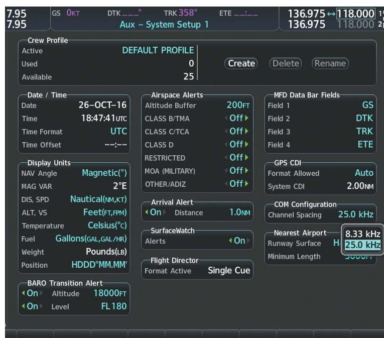
Figure 4-7 AUX – System Setup 1 Page
