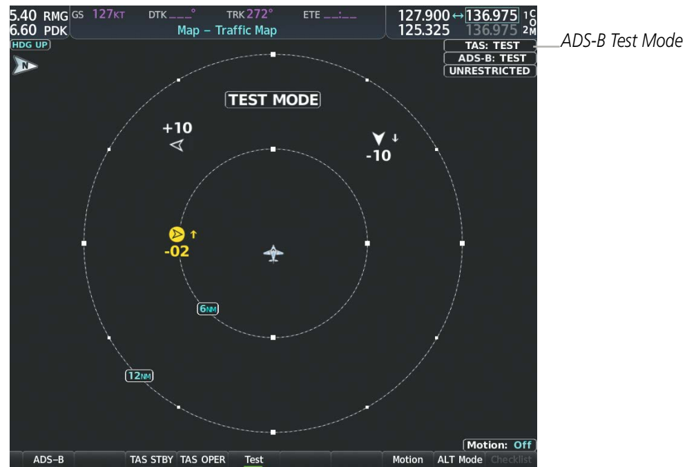
Figure 6-77 System Test in Progress with Test Pattern
