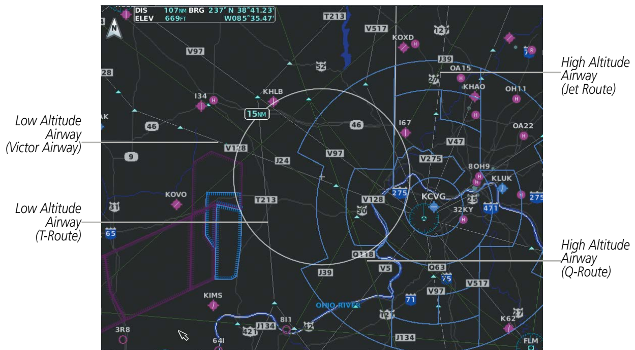
Figure 5-15 Airways on MFD Navigation Page
