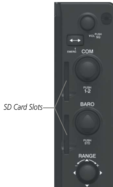
Figure 1-3 PFD/MFD Display Bezel SD Card Slots
