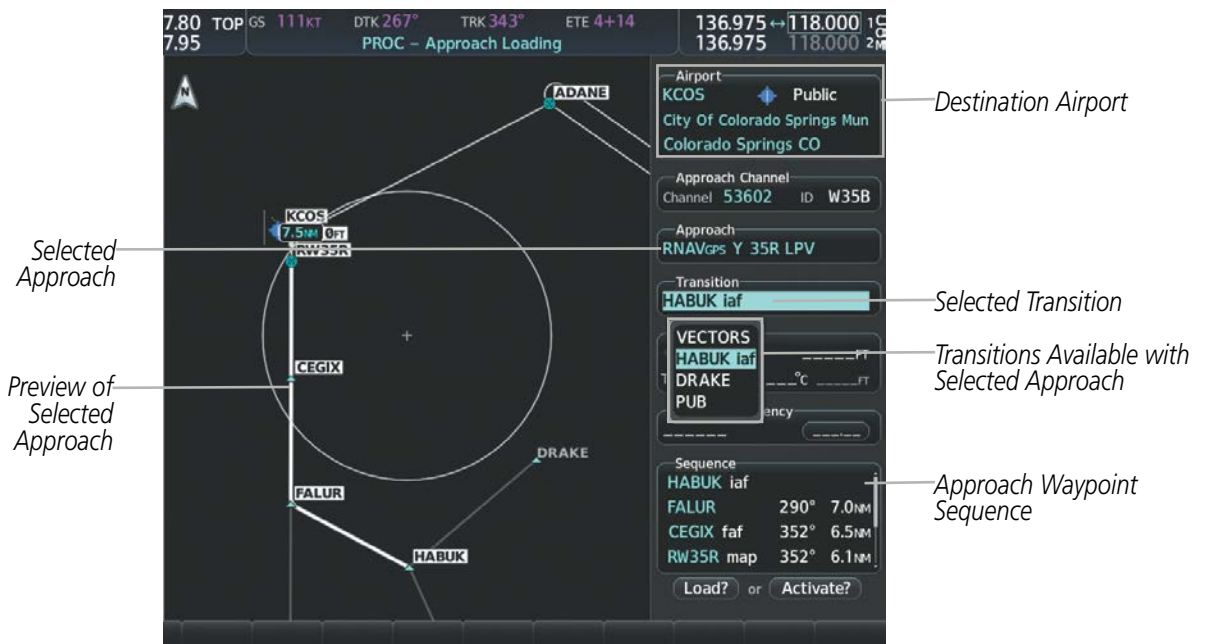
Figure 5-62 Approach Loading Page - Selecting the Transition
