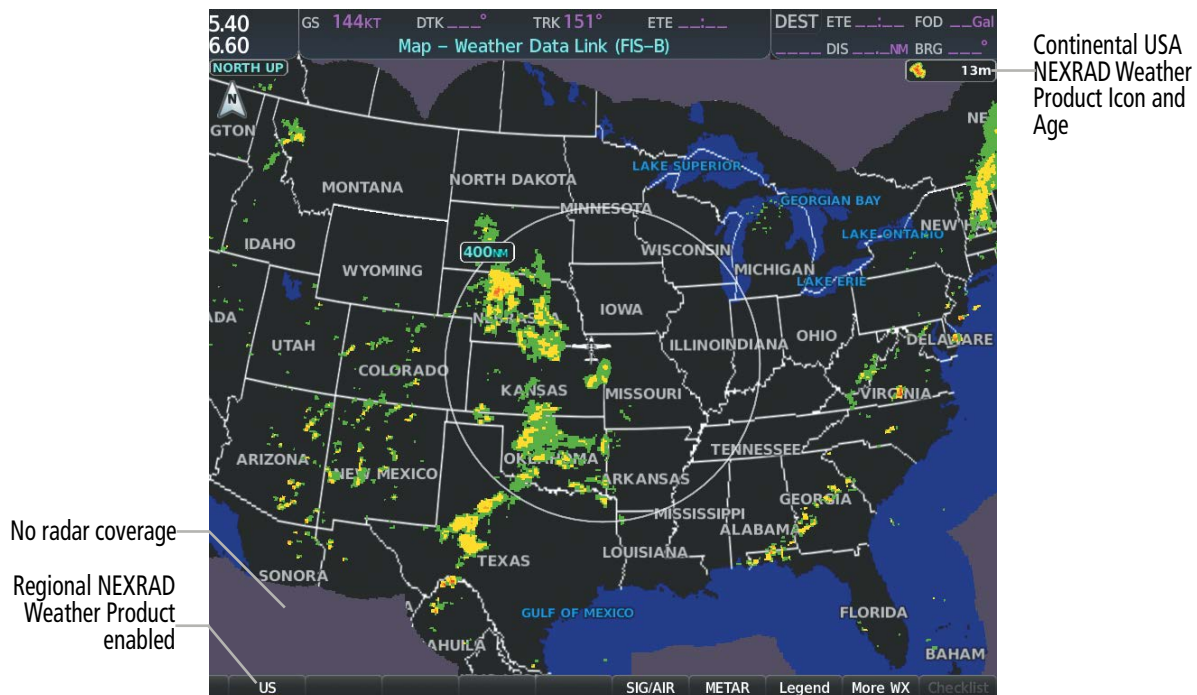
Figure 6-14 Continental US (CONUS) NEXRAD Weather Product on the 'Map - Weather Data Link (FIS-B)' Page
