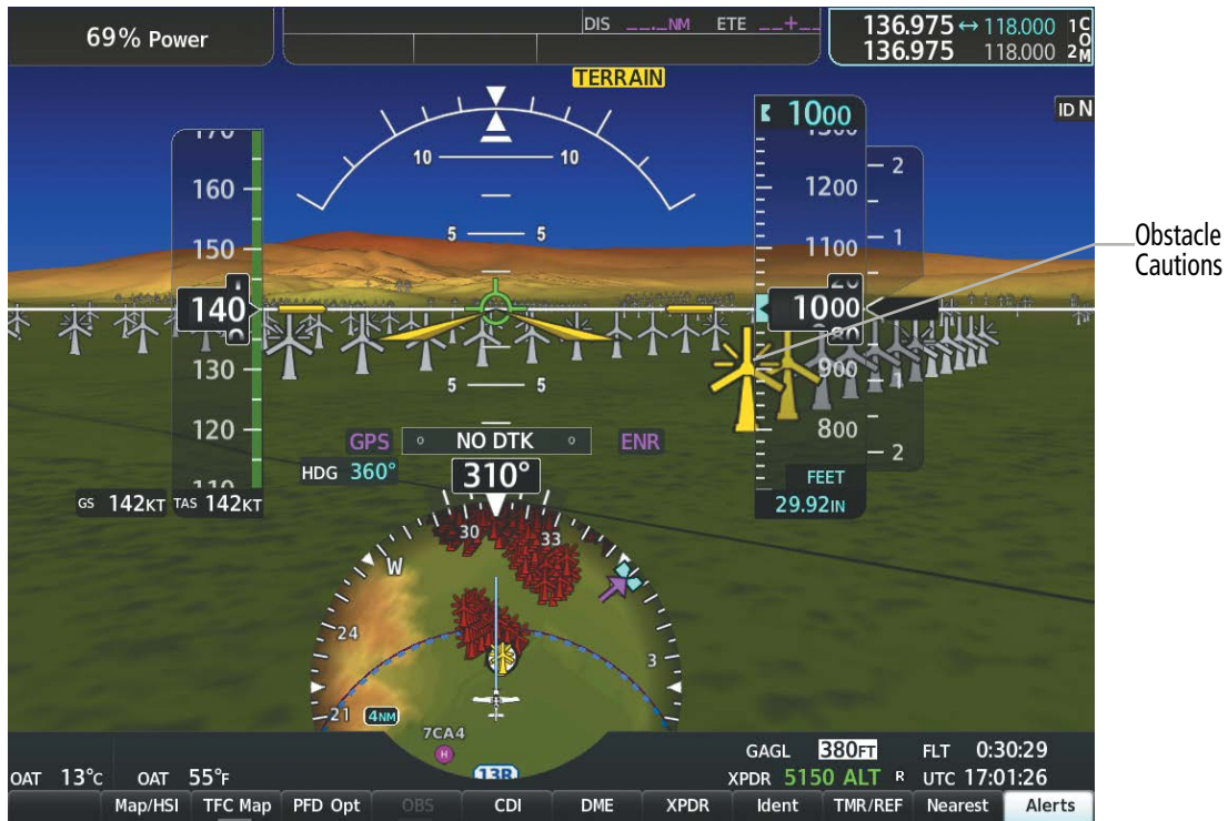
Figure 2-48 SVT with Obstacle Cautions
