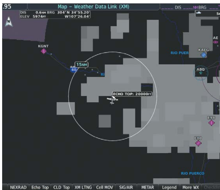
Figure 6-19 Echo Tops Weather Product on the 'Map - Weather Data Link (XM)' Page
