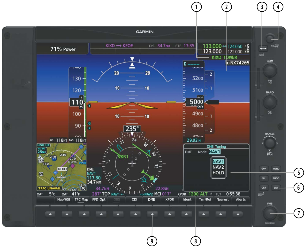
Figure 4-1 PFD Controls, COM Frequency Tuning Boxes, Transponder Code, and 'DME Tuning' Window
