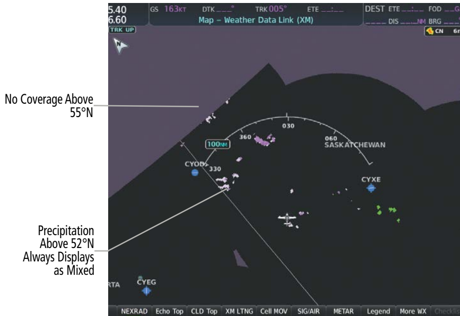
Figure 6-12 NEXRAD Weather Product on the 'Map - Weather Data Link (XM)' Page - Canada
