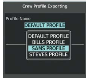
Crew Profile Exporting Window, Enter a Name to Use for Exported Profile
