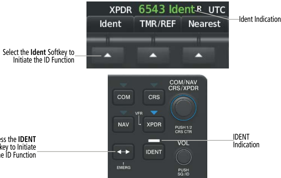
Figure 4-25 IDENT Softkey and Indication
