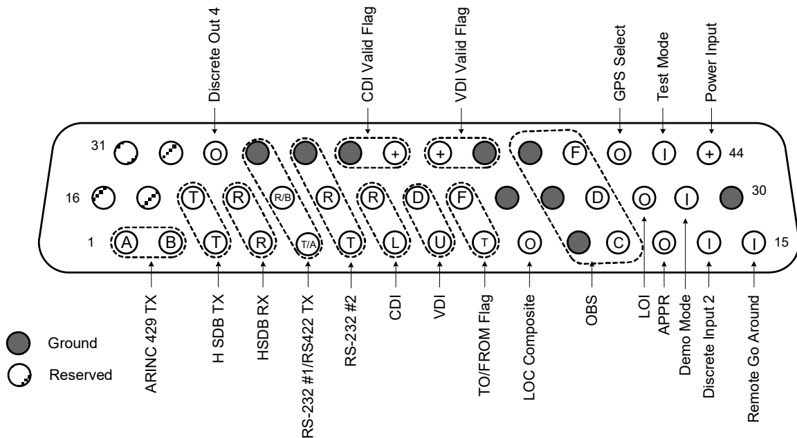
Figure 5-14 J3752 Connector (Looking at Unit)
