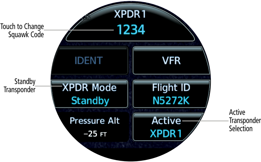
ADI - Transponder Control Display - Change Squawk Code
