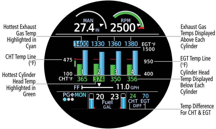
CHT/EGT - Four Cylinders - Bar Graph Example
