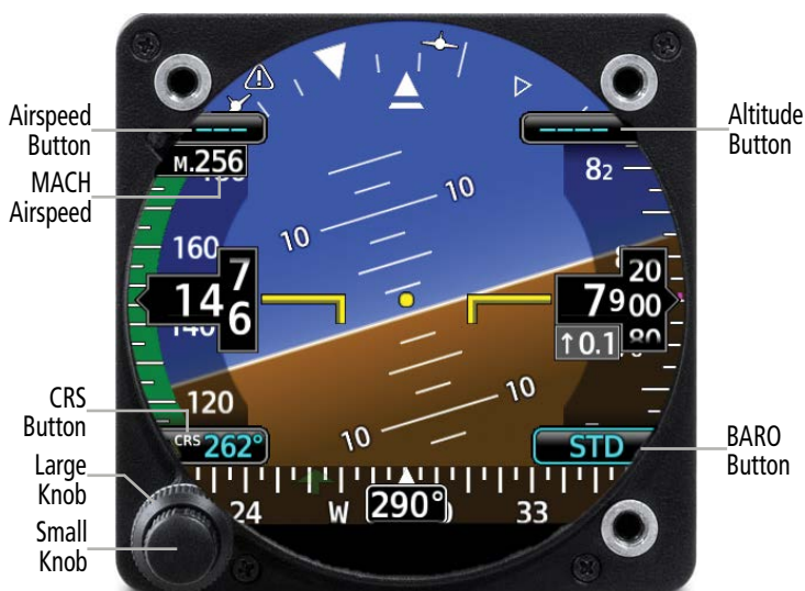
GI 275 Controls - Aircraft Symbol Change - MACH
