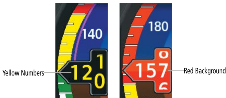
Airspeed Indicator - Approaching and Exceeding VNE
