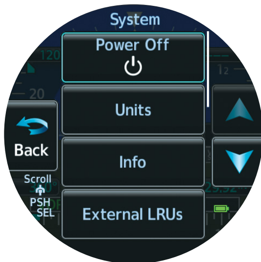
Battery - Power-Off Menu
