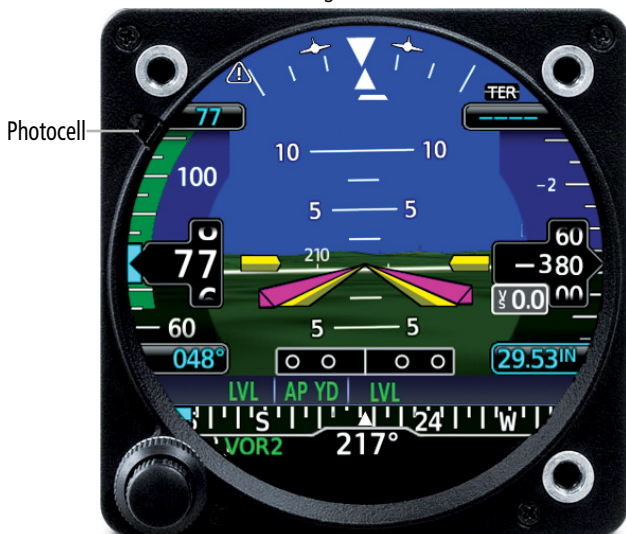
GI 275 Built-In Photocell
