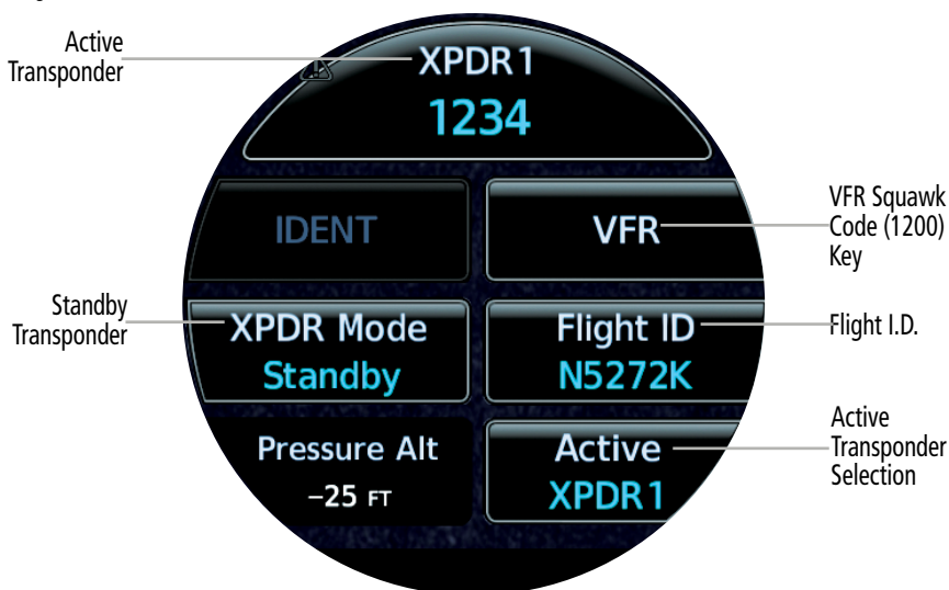
ADI - Transponder Control Display
