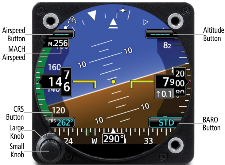
GI 275 Controls - Aircraft Symbol Change - MACH
