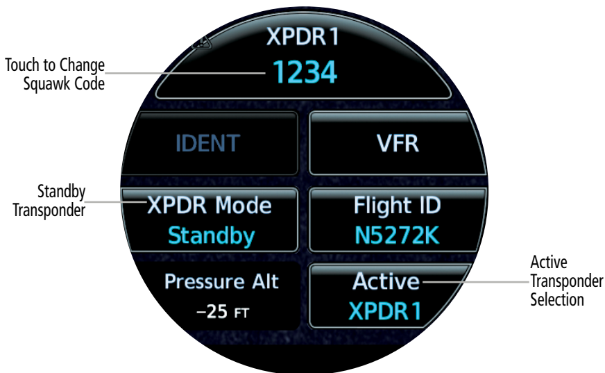
ADI - Transponder Control Display - Change Squawk Code
