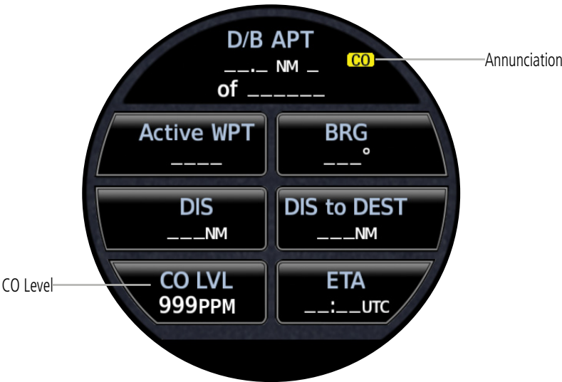
Garmin Carbon Monoxide Sensor - CO Level - Annunciation
