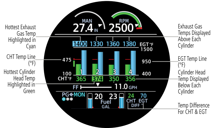
CHT/EGT - Four Cylinders - Bar Graph Example
