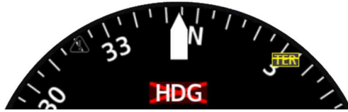
Figure 7- Top of the HSI when HDG failed (no GPS)
