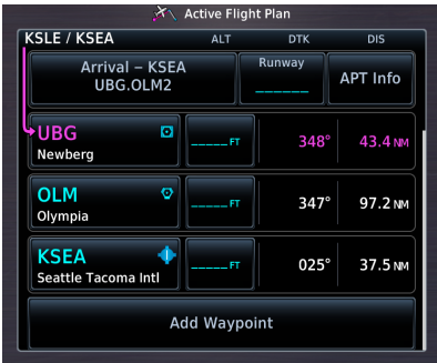
Active Flight Plan provides navigation to the airport waypoint when you defer runway selection.
