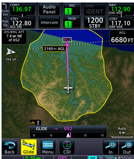
The GLIDE key replaces the Messages key when the Emergency page is not active.
