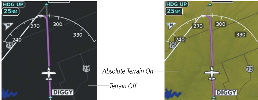
Figure 5-14 PFD Inset Map - Absolute Terrain Data
