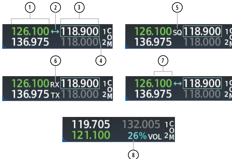
Figure 4-3 COM Tuning Box Indications
