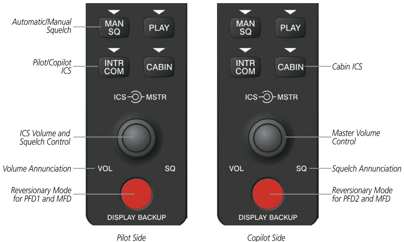
Figure 4-19 Audio Panel Controls
