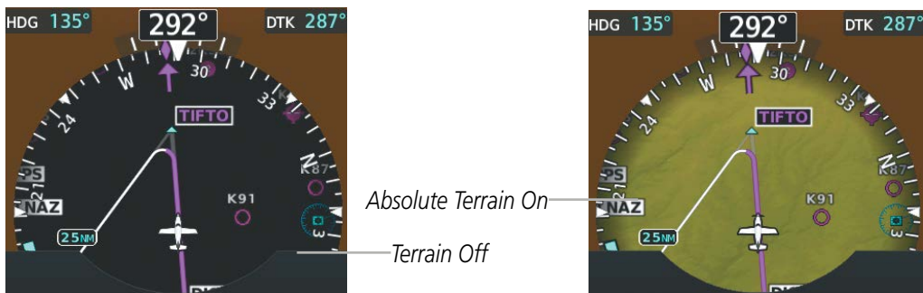
Figure 5-15 HSI Map - Absolute Terrain Data
