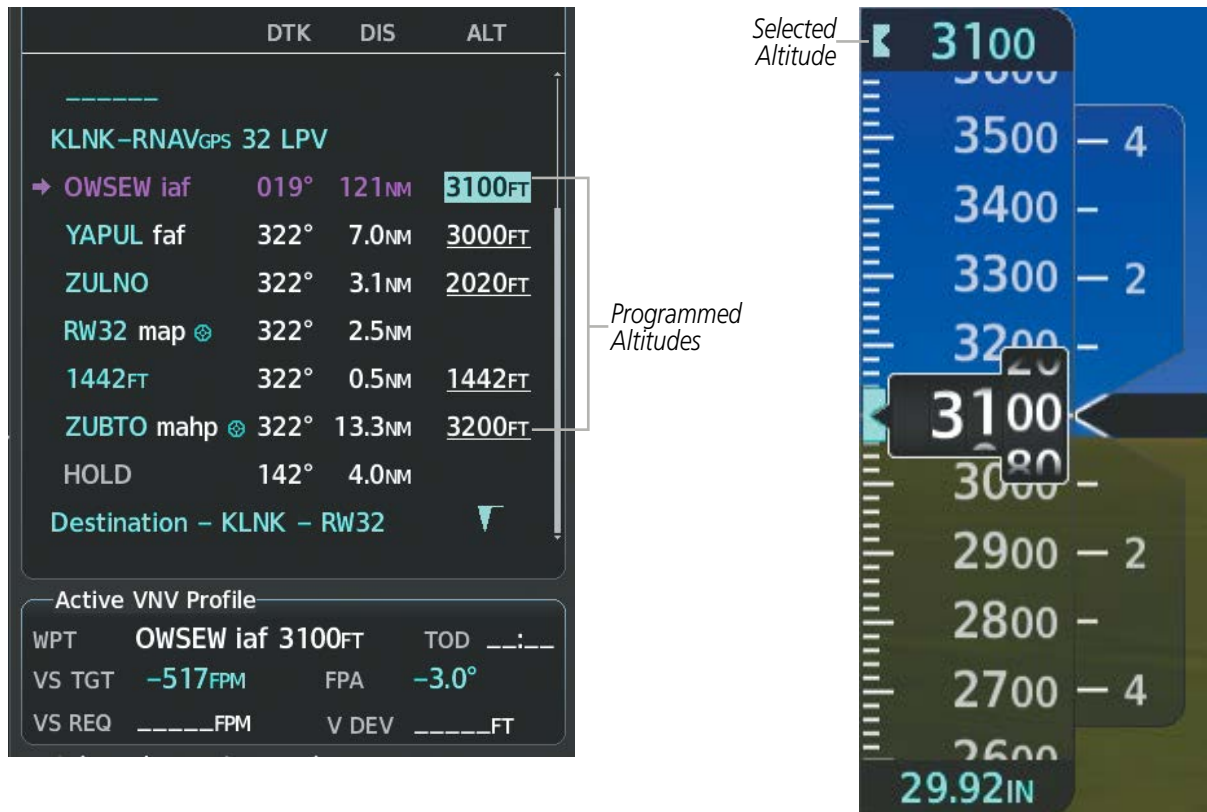
Figure 2-50 Programmed and Selected Altitude
