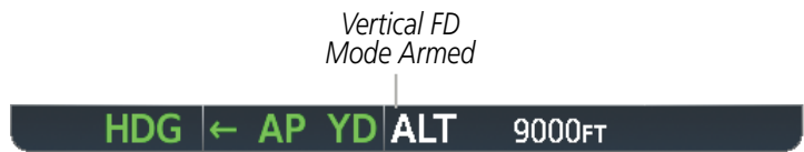
Figure 7-39 Vertical Flight Director Mode Armed
