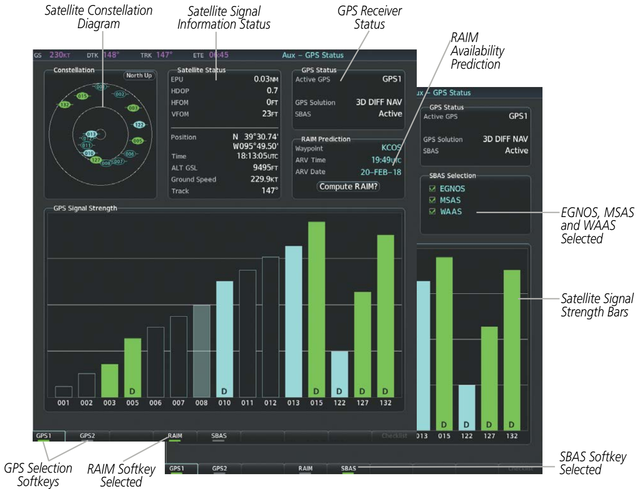
Figure 1-11 GPS Status Page (RAIM or SBAS Selected)
