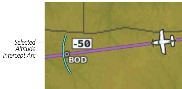
Figure 5-18 Navigation Map - Range to Altitude Arc
