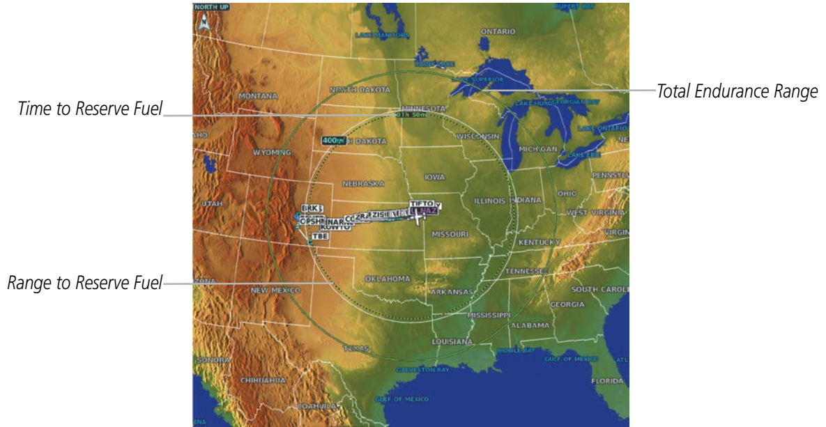
Figure 5-21 Navigation Map - Fuel Range Ring
