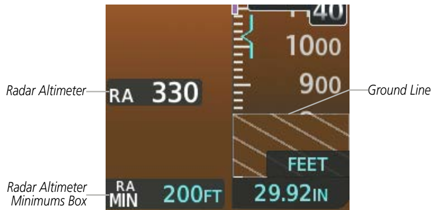
Figure 2-21 Altimeter Displaying the Ground Line (RAD ALT)
