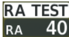
Figure 2-23 Radar Altimeter with Test Annunciation
