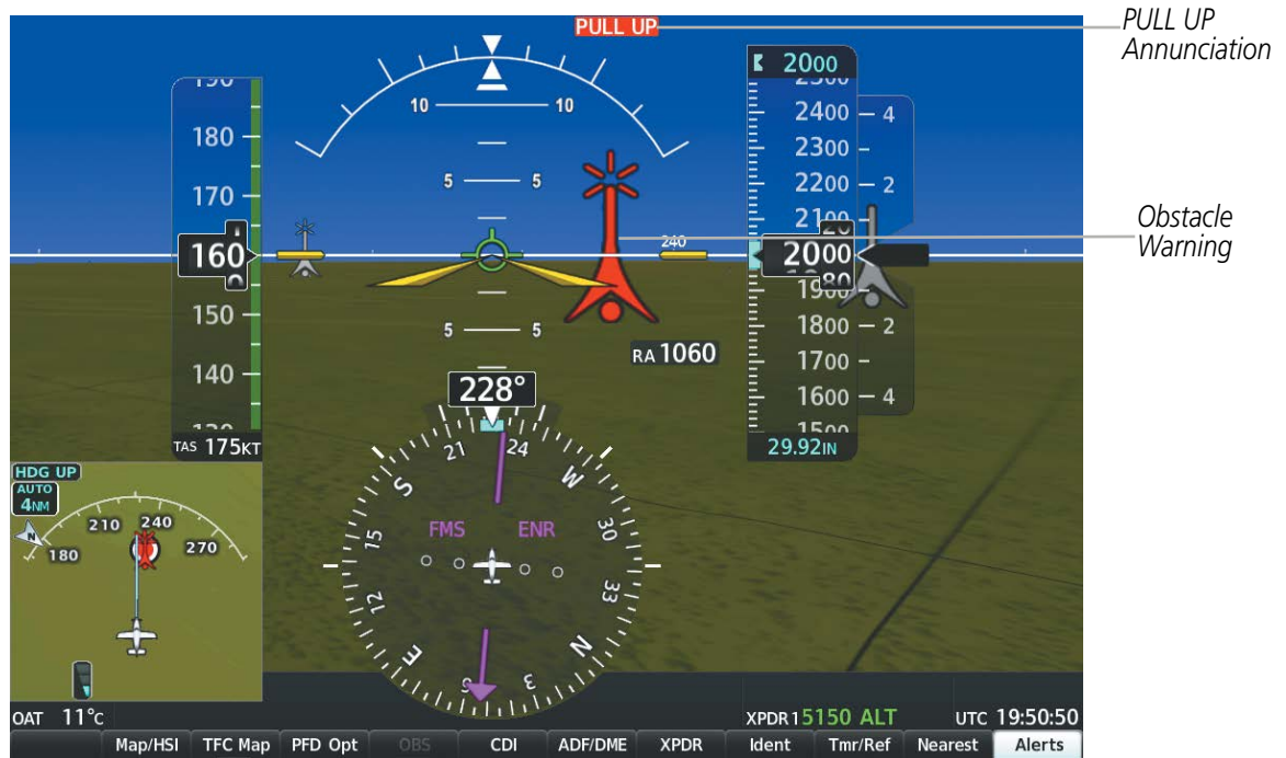
Figure 2-55 SVT Obstacle Warning
