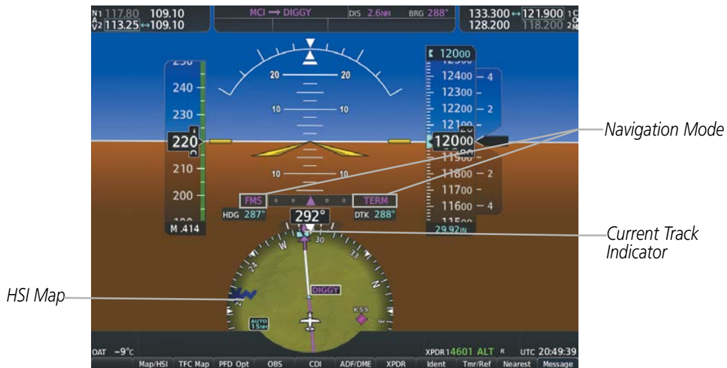
Figure 5-2 GPS Navigation Information on the PFD HSI Map
