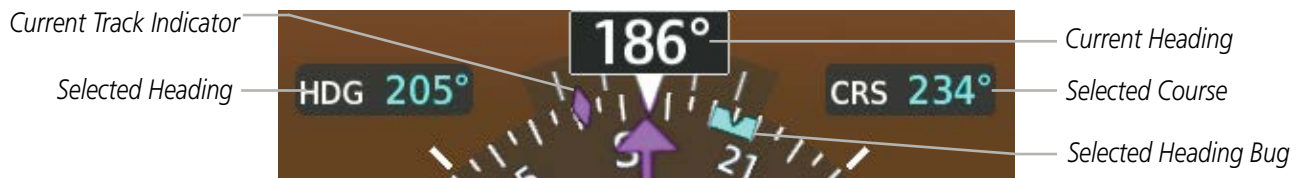
Figure 2-26 Heading and Course Indications
