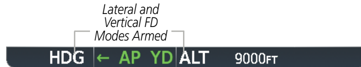
Figure 7-37 Lateral and Vertical Flight Director Modes Armed
