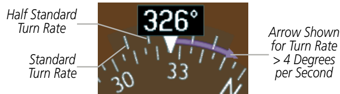
Figure 2-37 Turn Rate Indicator and Trend Vector
