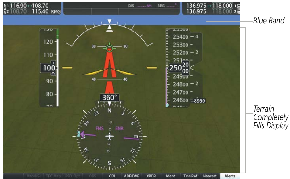
Figure 2-61 Blue Sky Bar with Full Display Terrain
