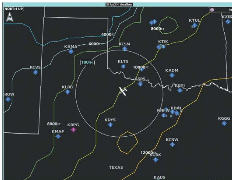
Figure 6-44 Freezing Level Weather Product
