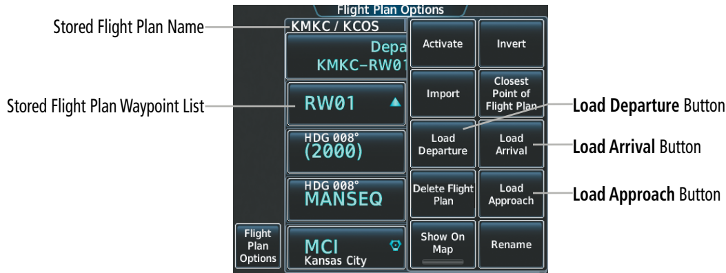
Figure 5-125 Loading a Procedure into a Stored Flight Plan - 'Flight Plan Options' Window
