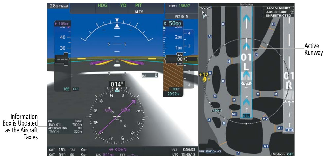
Figure 8-3 SurfaceWatch Information on the PFD
