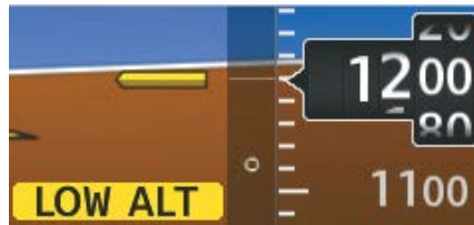
Figure 2-47 Low Altitude on GPS SBAS Approach
