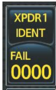
Figure 4-68 Transponder Fail Indication
