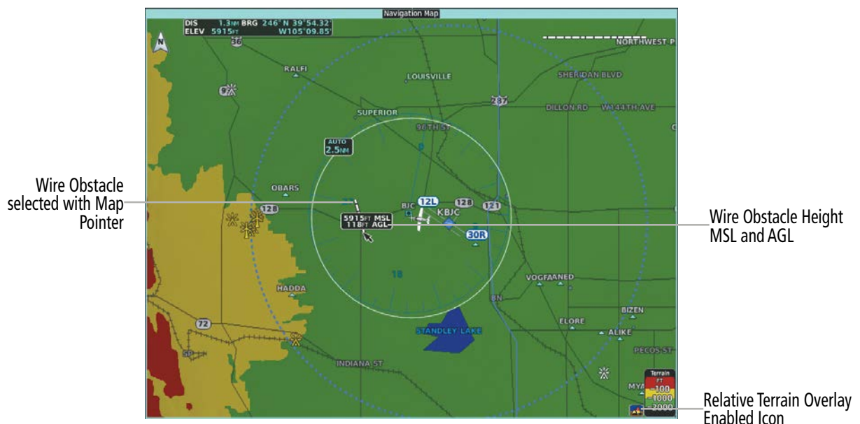
Figure 6-98 Using the Map Pointer to get Wire Obstacle Height 'Navigation Map' Pane
