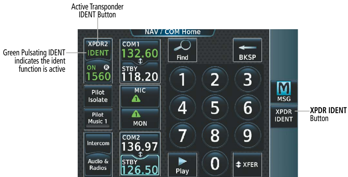
Figure 4-52 Transponder IDENT Controls
