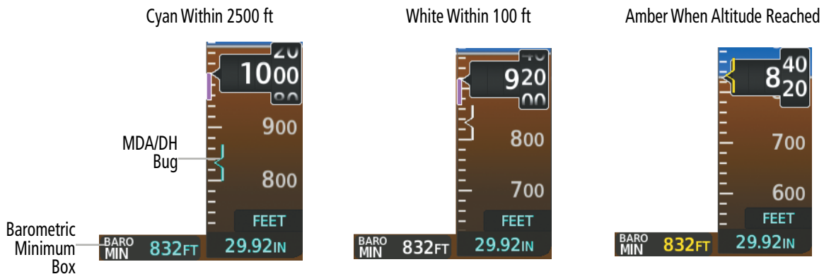
Figure 2-48 Barometric MDA/DH Alerting Visual Annunciations
