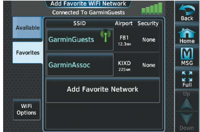
Figure 8-96 Connected Network Indication
