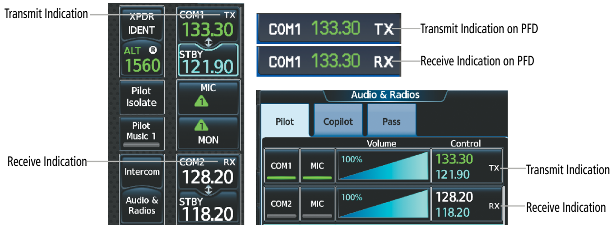
Figure 4-4 COM Radio Transmit and Receive Indications
