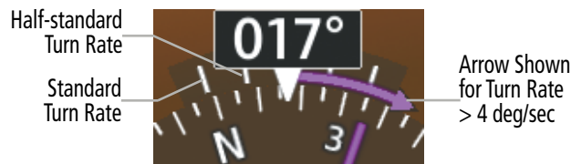
Figure 2-21 Turn Rate Indicator and Trend Vector
