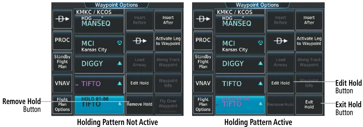
Figure 5-98 Removing a User Defined Holding Pattern at an Active Flight Plan Waypoint
