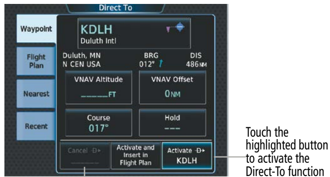
Figure 1-6 Subdued Buttons on Touchscreen Controller
