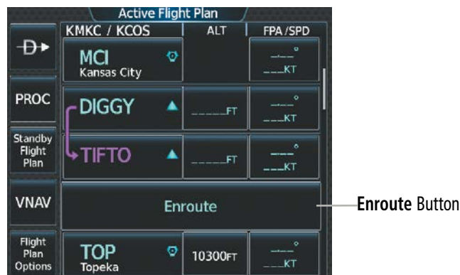
Figure 5-67 Adding a Waypoint to the beginning of the Enroute Segment of the Flight Plan
