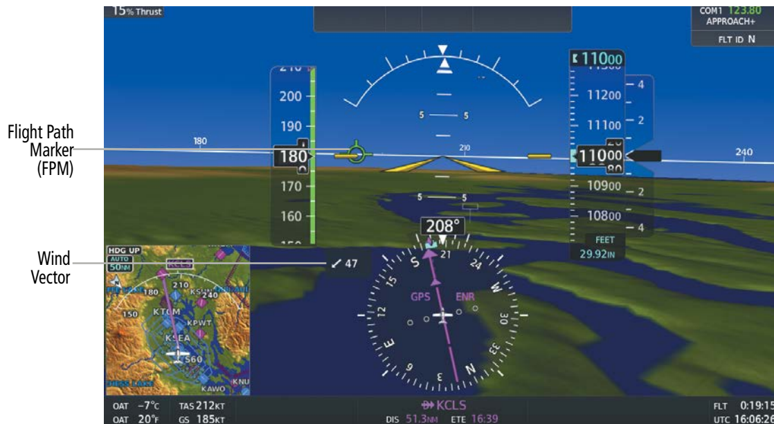
Figure 2-36 Flight Path Marker Position is Affected by Wind
