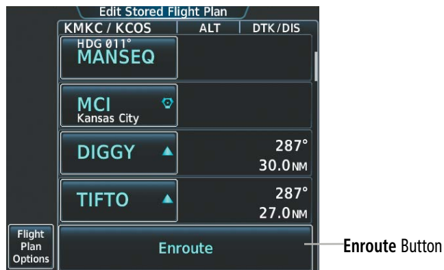
Figure 5-70 Edit Stored Flight Plan - Adding a Waypoint to the beginning of the Enroute Segment of the Flight Plan
