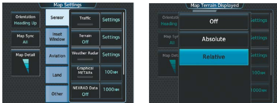
Figure 6-90 Enabling Relative Terrain for the Profile View Inset Window and 'Navigation Map' Pane
