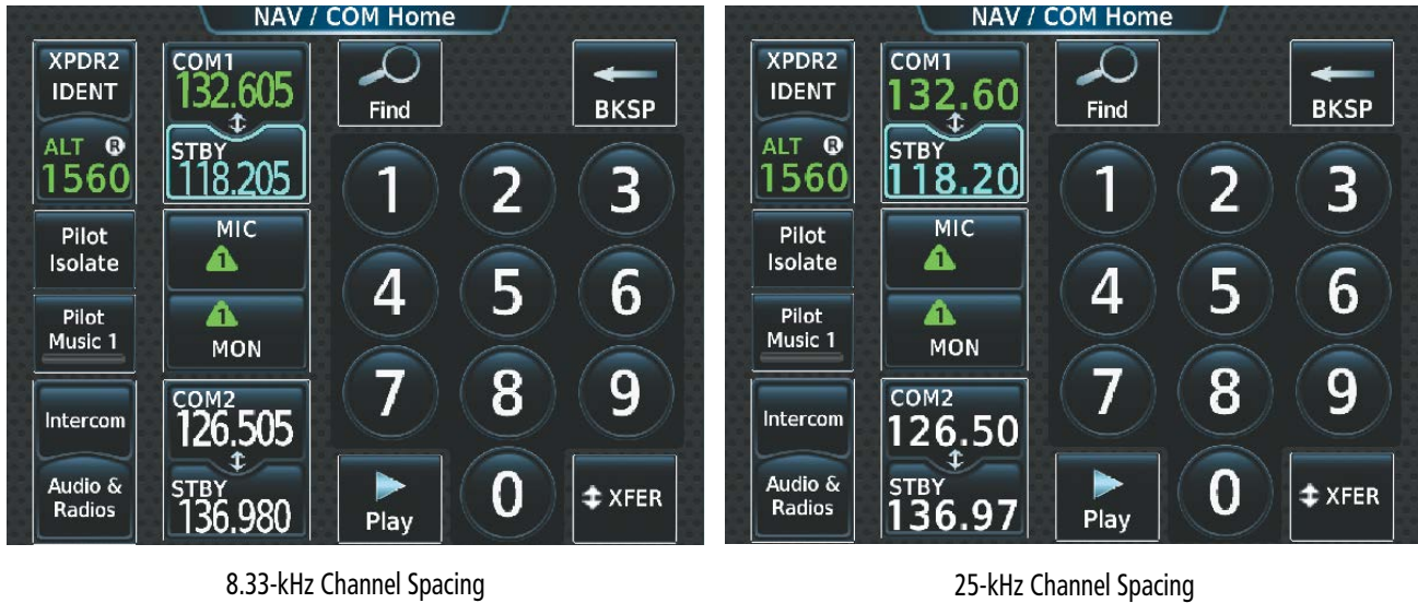
Figure 4-17 COM Channel Spacing
