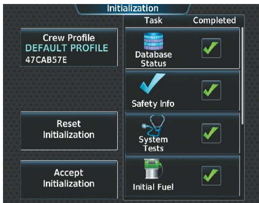
Figure 1-26 System Initialization Completed Tasks
