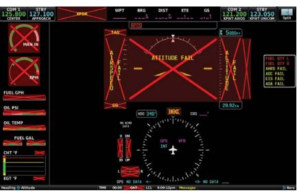
**G3X Touch System Failure Annunciations**
