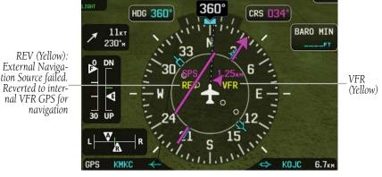
**External GPS Navigator Failure**
