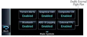
**External Flight Plan Enabled (Configuration Mode)**
