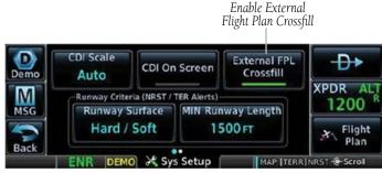
External Flight Plan Crossfill Enabled (Normal Mode)
