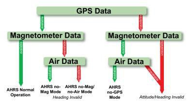
Loss of GPS, magnetometer, or air data inputs is communicated to the pilot by message advisory alerts. Any failure of the internal AHRS inertial sensors results in loss of attitude and heading information (indicated by red 'X' flags over the corresponding flight instruments). If the G3X Touch senses the magnetic heading measurement is valid, but possibly outside of the internal accuracy limits, the numeric heading value on the PFD is displayed in yellow.
