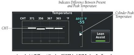
Lean Assist (Different Number Of EGT And CHT Probes Configured And **Less Than Four Cylinders Configured)**
