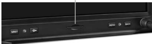
SD Card Slot - GDU™ 460 (10.6 inch)
