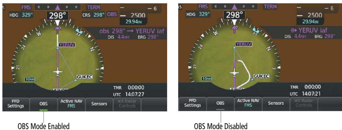
Figure 2-36 Omni-bearing Selector (OBS) Mode on the HSI Map
