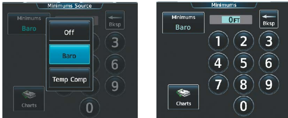
Figure 2-52 Baro and Temp Comp Minimum Altitude Alerting
