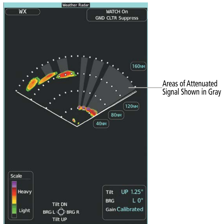
Figure 6-92 Horizontal Scan with WATCH® Enabled
