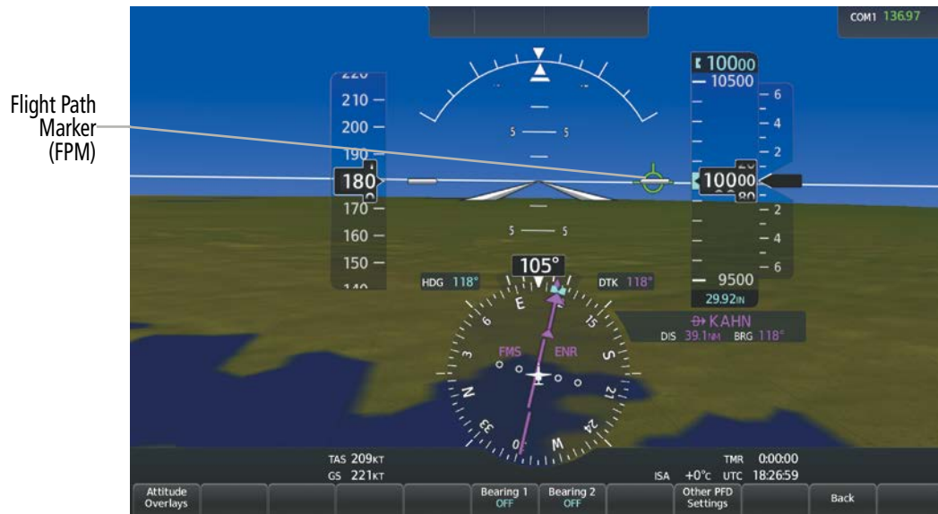
Figure 2-40 Flight Path Marker Position is Affected by Wind
