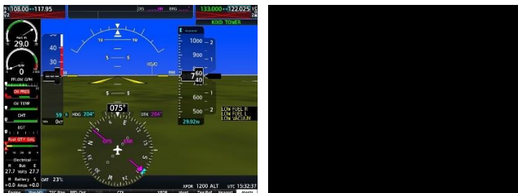
Figure 2-7, Automatic Reversion with MFD failure
