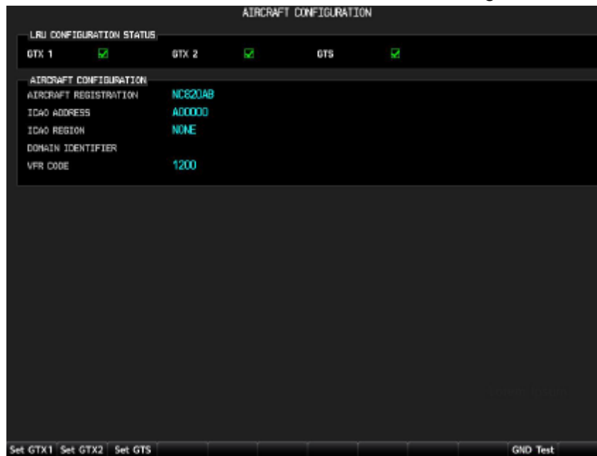
Figure 7-2, GTX Ground Test Mode Softkey
