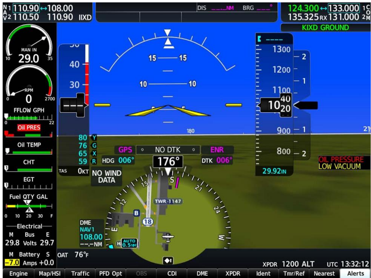
Figure 9-4, GDU Reversionary Mode
