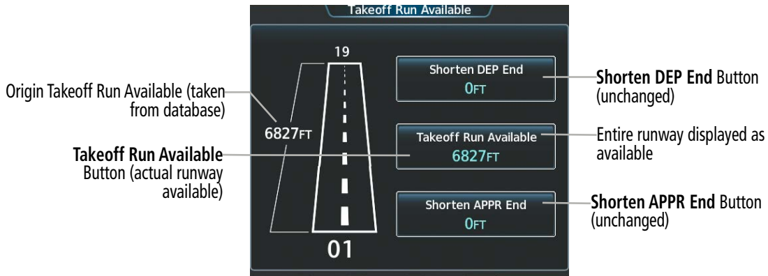
Figure 5-175 Takeoff Run Available – Normal
