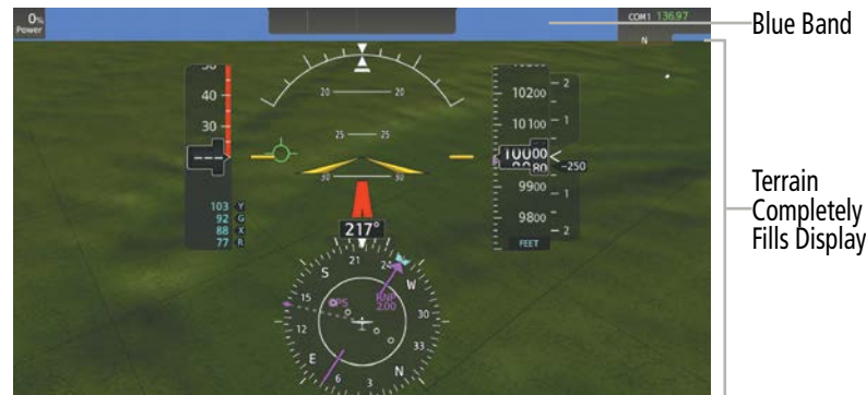
Figure 2-61 Blue Sky Bar with Full Display Terrain
