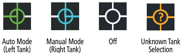
Figure 3-17 Ice Protection Tank Selection Status Icons
