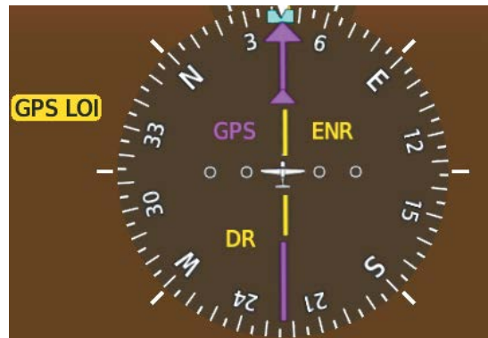
Figure 2-58 Abnormal GPS Condition Annunciations
