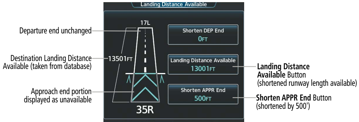
Figure 5-185 Landing Distance Available – Shortened Approach End
