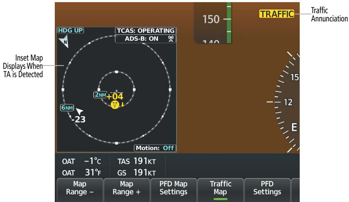
Figure 6-110 Traffic Annunciation (PFD)
