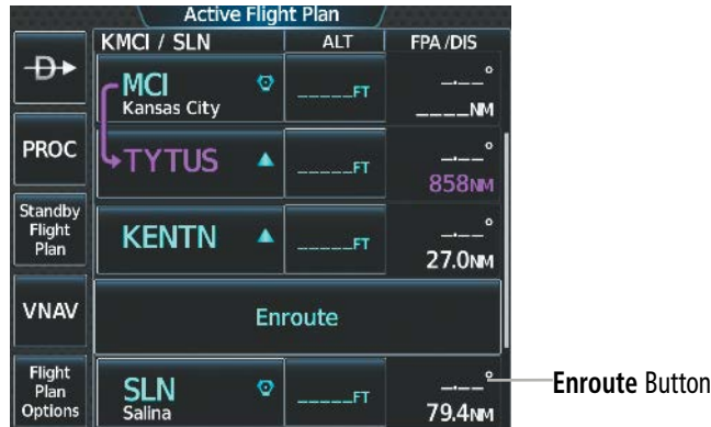
Figure 5-86 Active Flight Plan – Adding a Waypoint to the beginning of the Enroute Segment of the Flight Plan
