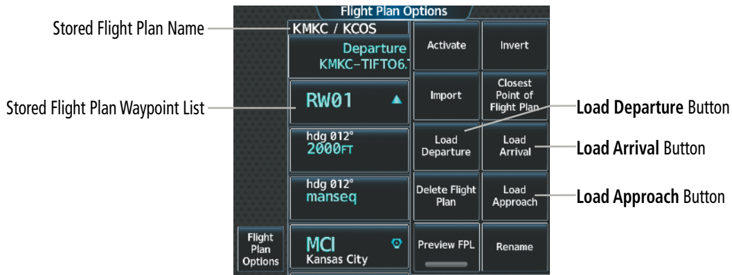
Figure 5-141 Loading a Procedure into a Stored Flight Plan – 'Flight Plan Options' Window
