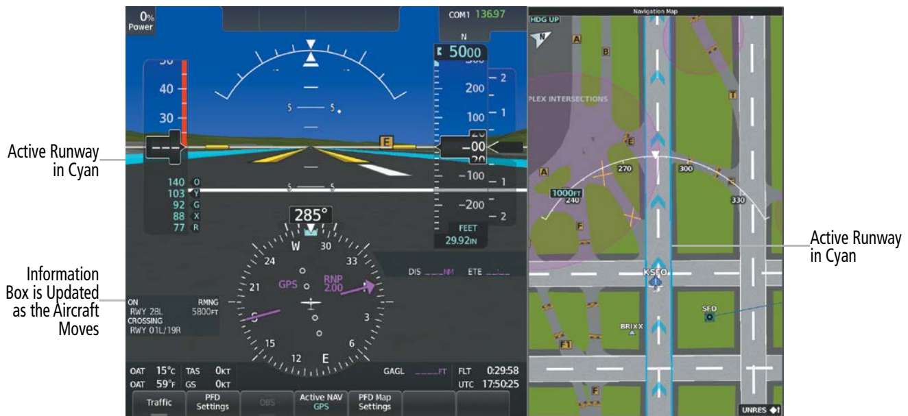
Figure 8-4 SurfaceWatch Information on the PFW
