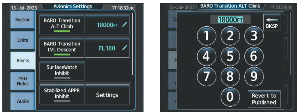
Figure 2-10 BARO Transition Alert
