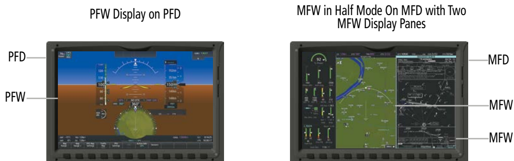
Figure 1-5 PFW and MFW Displays on PFD and MFD in Normal and Half Mode
