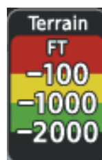
Figure 6-87 Relative Terrain Legend
