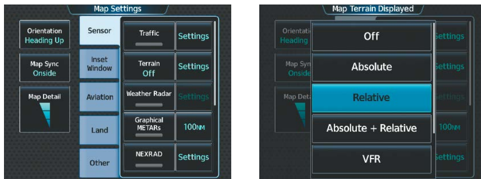
Figure 6-83 Enabling Relative Terrain for the Profile View Inset Window and 'Navigation Map' Pane
