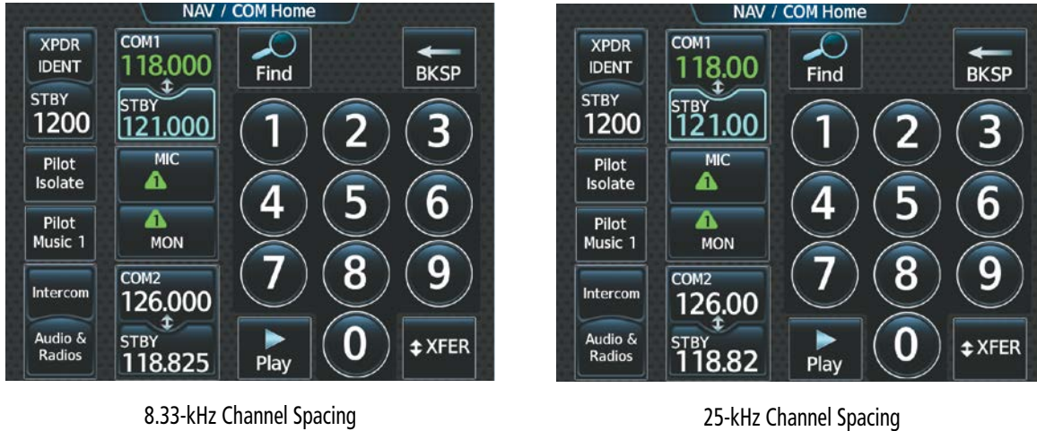
Figure 4-19 COM Channel Spacing
