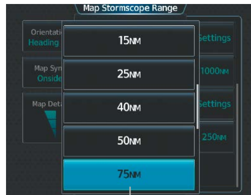
Touch to select maximum map range for Stormscope information to be displayed on selected Navigation Map Pane
