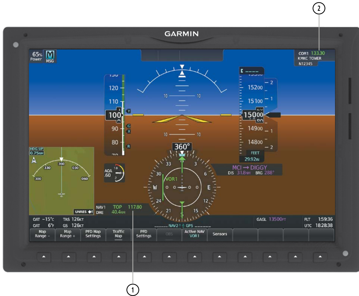
Figure 4-2 PFD Active NAV Window, Active COM Frequency Box
