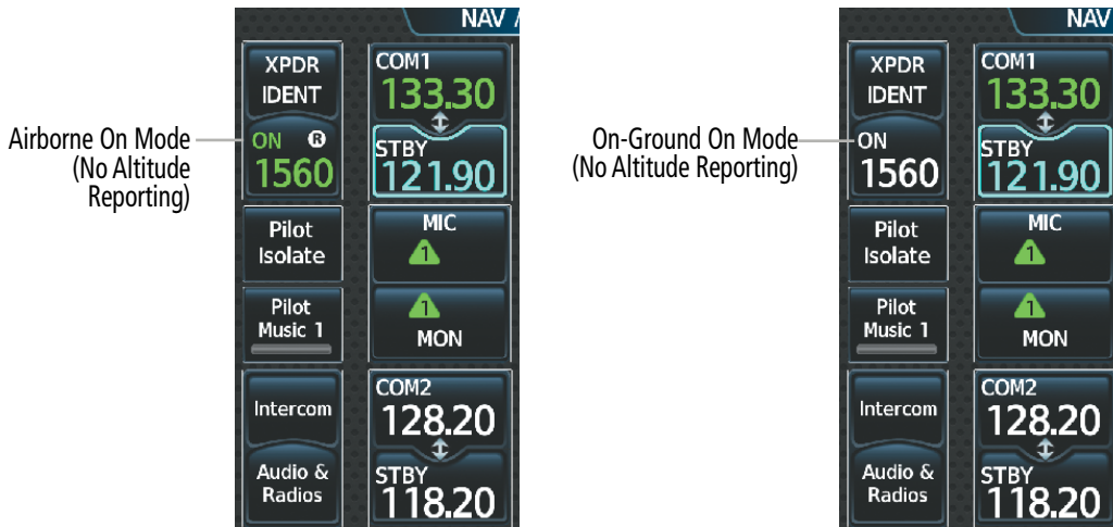
Figure 4-44 On Mode Indications
