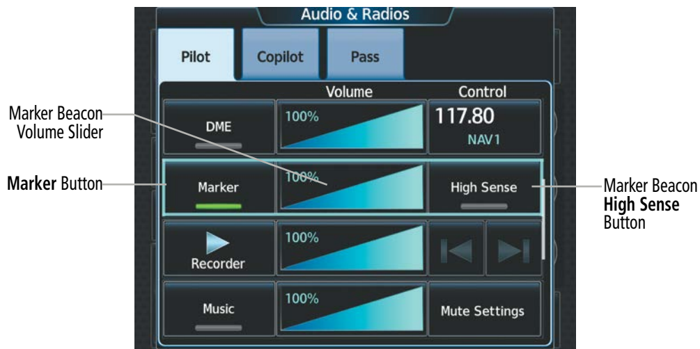
Figure 4-37 Marker Beacon Controls
