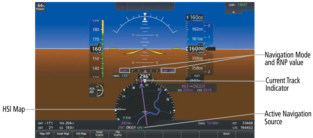
Figure 5-2 GPS Navigation Information on the PFW HSI Map
