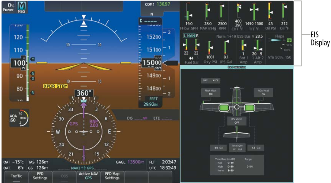
Figure 3-20 EIS (Reversionary Mode)
