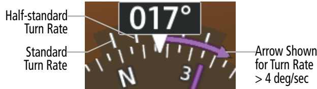
Figure 2-19 Turn Rate Indicator and Trend Vector
