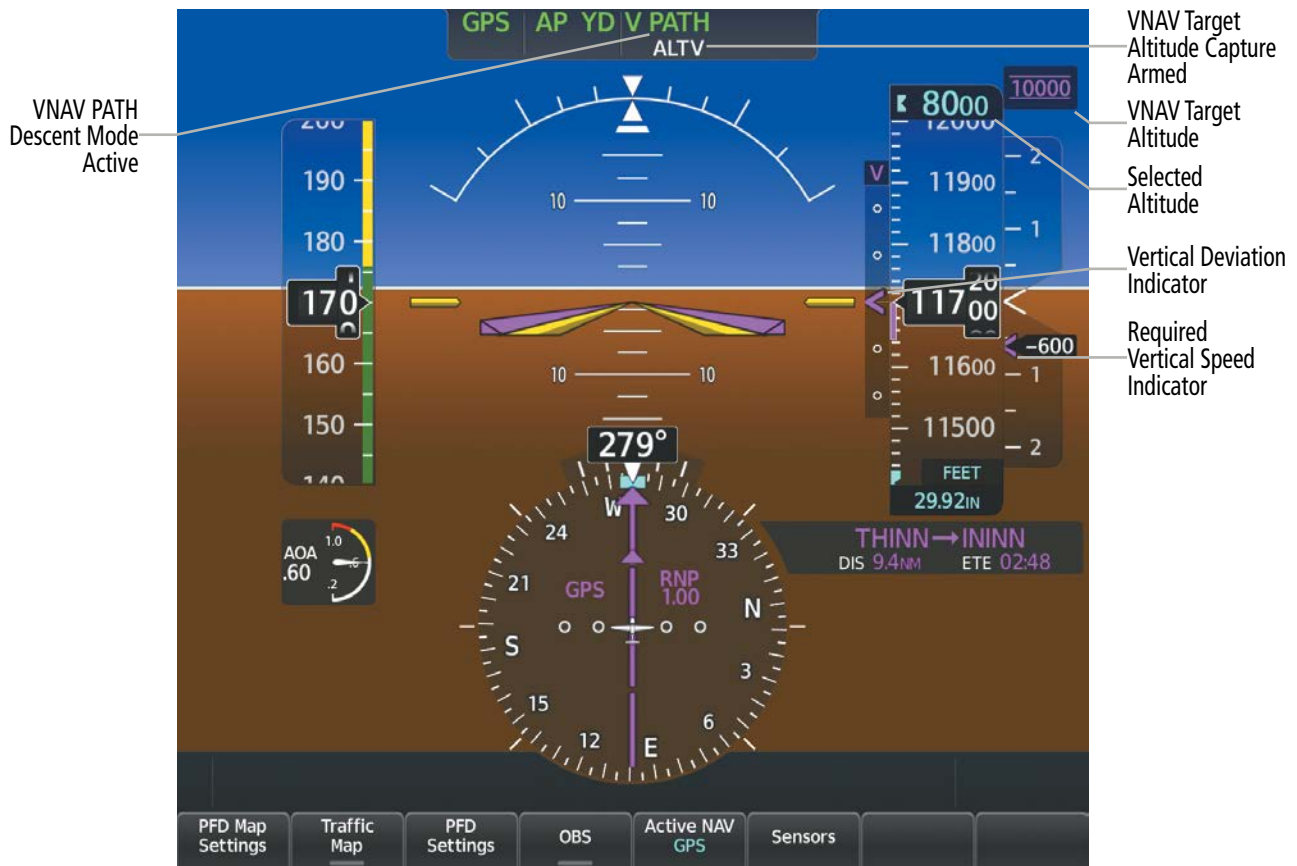
Figure 7-16 VNAV PATH Descent Mode
