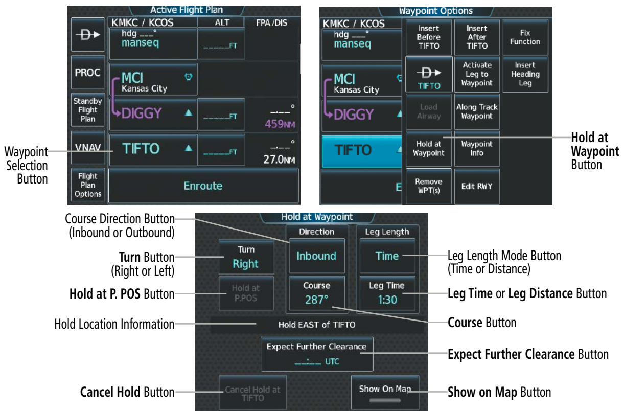
Figure 5-123 Creating a User Defined Holding Pattern at an Active Flight Plan Waypoint
