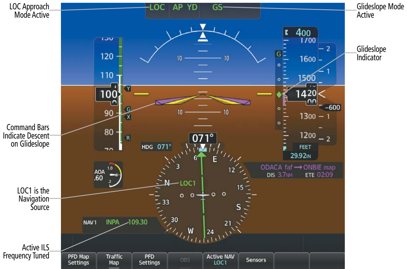
Figure 7-30 Glideslope Mode Active
