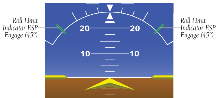
ESP Roll Engagement Indication (ESP NOT Engaged)
