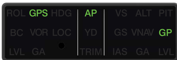
GI 285 AFCS Annunciator Panel Annunciating Glidepath Mode
