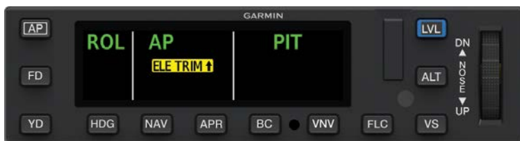
GMC 605C-FLC AFCS Mode Controller with Color Display Mistrim Indication
