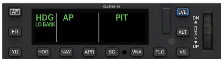
GMC 605C-FLC AFCS Mode Controller with Color Display Annunciating Low Bank Mode
