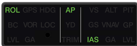
GI 285 AFCS Annunciator Panel Annunciating Indicated Airspeed Mode
