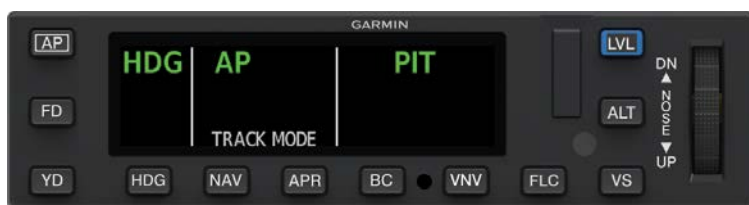
GMC 605C-FLC AFCS Mode Controller with Color Display Annunciating Reversionary GPS Track Mode
