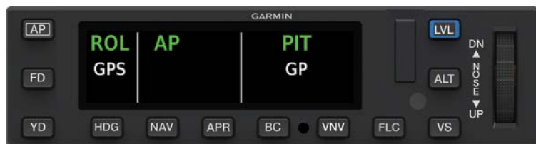
GMC 605C-FLC AFCS Mode Controller with Color Display Annunciating GPS Approach Mode Armed
