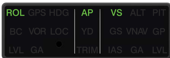
GI 285 AFCS Annunciator Panel Annunciating Vertical Speed Mode
