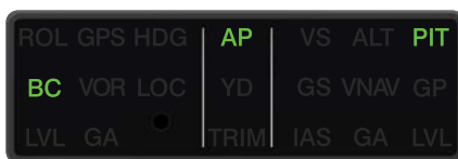
GI 285 AFCS Annunciator Panel Annunciating Backcourse Mode
