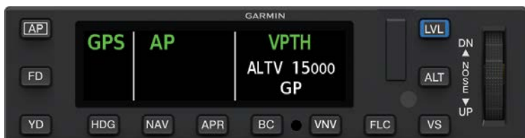
GMC 605C-FLC AFCS Mode Controller with Color Display Annunciating VPTH/GP Mode
