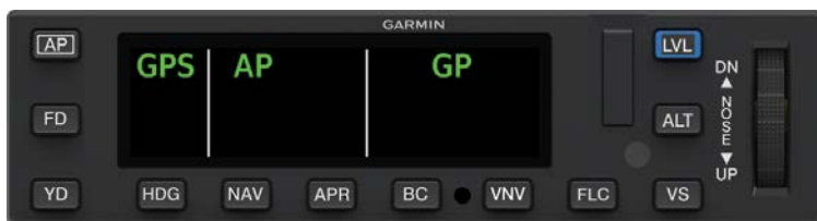
GMC 605C-FLC AFCS Mode Controller with Color Display Annunciating Glidepath Mode
