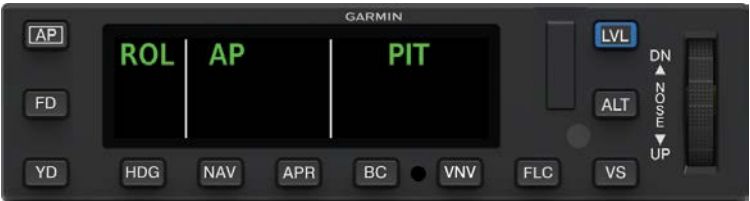
GMC 605C-FLC AFCS Mode Controller with Color Display Annunciating Roll Hold Mode
