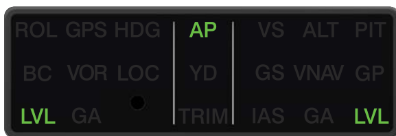
GI 285 AFCS Annunciator Panel Annunciating Level Mode
