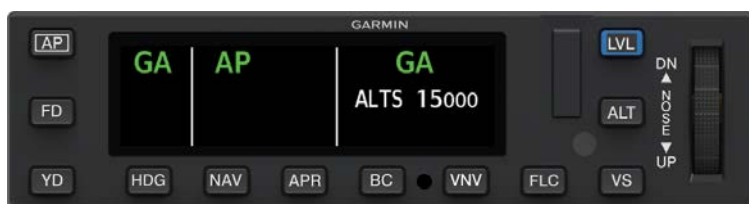
GMC 605C-FLC AFCS Mode Controller with Color Display Annunciating Go Around Mode
