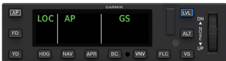
GMC 605C-FLC AFCS Mode Controller with Color Display Annunciating Glideslope Mode
