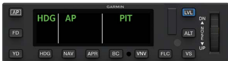
GMC 605C-FLC AFCS Mode Controller with Color Display Annunciating Heading Mode
