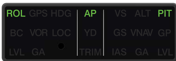
GI 285 AFCS Annunciator Panel Annunciating Roll Hold Mode
