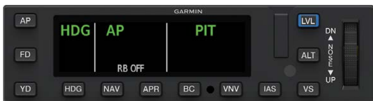
GMC 605C-IAS AFCS Mode Controller with Color Display Annunciating Smart Rudder Bias Off (RB OFF)
