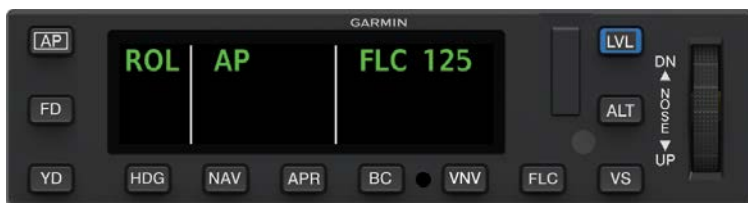
GMC 605C-FLC AFCS Mode Controller with Color Display Annunciating Flight Level Change Mode
