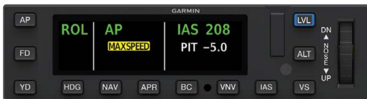
GMC 605C-IAS AFCS Mode Controller with Color Display Overspeed Indication
