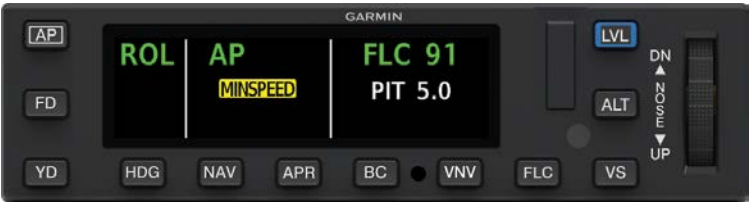
GMC 605C-FLC AFCS Mode Controller with Color Display Underspeed Indication (Non-Altitude Critical Mode)
