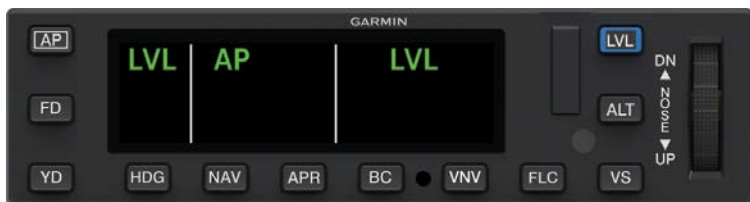
GMC 605C-FLC AFCS Mode Controller with Color Display Annunciating Level Mode
