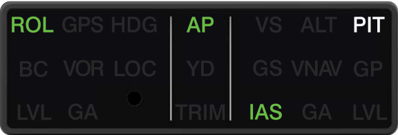
GI 285 AFCS Annunciator Panel Overspeed Indication
