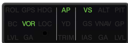
GMC 605C-FLC AFCS Mode Controller with Color Display Annunciating Various Approach Modes
