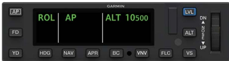
GMC 605C-FLC AFCS Mode Controller with Color Display Annunciating Alt Hold Mode
