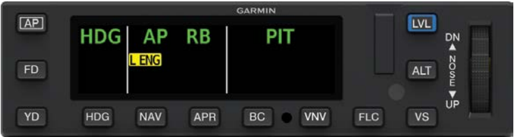
GMC 605C-IAS AFCS Mode Controller with Color Display Annunciating Smart Rudder Bias Active (Left Engine)
