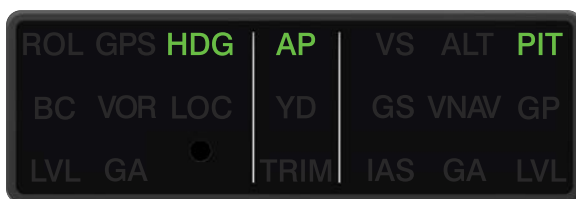
GI 285 AFCS Annunciator Panel Annunciating Heading Mode
