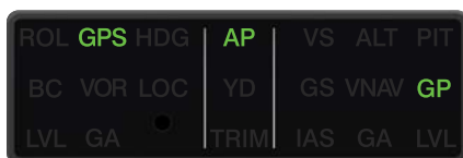
GI 285 AFCS Annunciator Panel Annunciating Various Approach Modes
