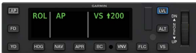
GMC 605C-FLC AFCS Mode Controller with Color Display Annunciating Vertical Speed Mode
