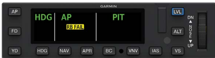
GMC 605C-IAS AFCS Mode Controller with Color Display Annunciating Smart Rudder Bias Fail (RB FAIL)
