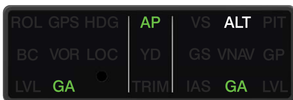
GI 285 AFCS Annunciator Panel Annunciating Go Around Mode
