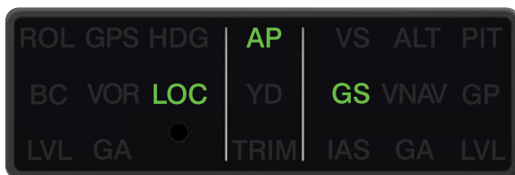
GI 285 AFCS Annunciator Panel Annunciating Glideslope Mode
