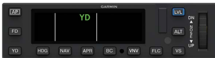
GMC 605C-FLC AFCS Mode Controller with Color Display Yaw Damper Indication
