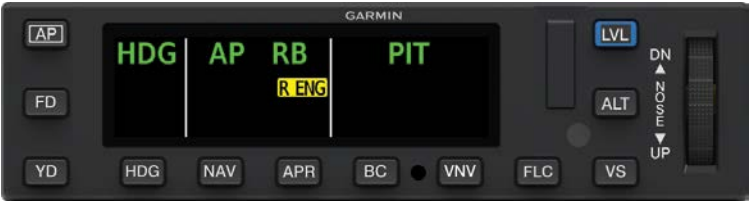
GMC 605C-IAS AFCS Mode Controller with Color Display Annunciating Smart Rudder Bias Active (Right Engine)
