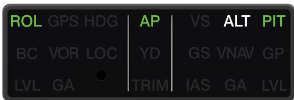
GI 285 AFCS Annunciator Panel Annunciating Pitch Mode
