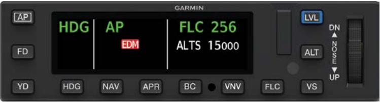
GMC 605C-16 AFCS Mode Controller with Color Display (-16 Model) Annunciating Emergency Decent Mode (Active)
