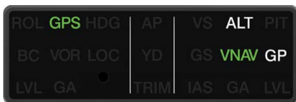
GI 285 AFCS Annunciator Panel Annunciating VNAV/GP Mode
