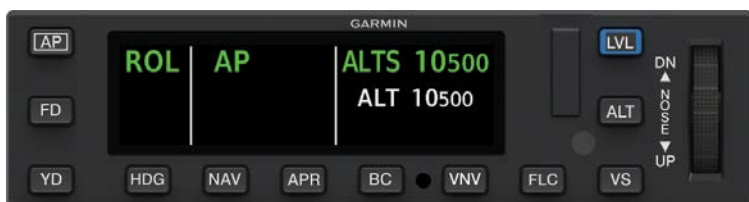
GMC 605C-FLC AFCS Mode Controller with Color Display Annunciating Selected Altitude Capture Mode
