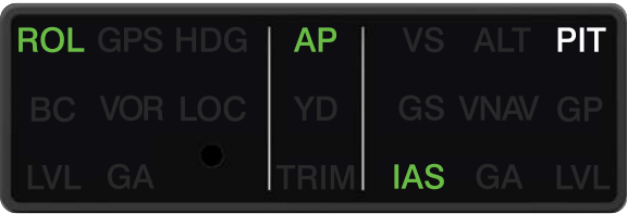
GI 285 AFCS Annunciator Panel Underspeed Indication (Non-Altitude Critical Mode)
