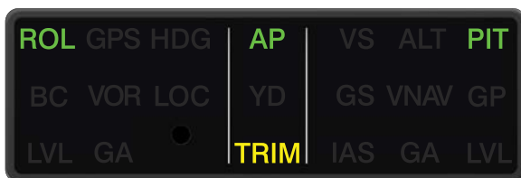
GI 285 AFCS Annunciator Panel Mistrim Indication
