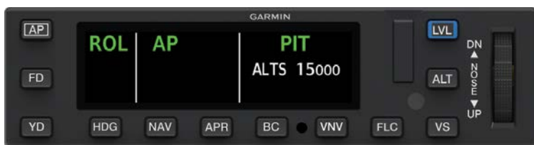
GMC 605C-FLC AFCS Mode Controller with Color Display Annunciating Pitch Mode
