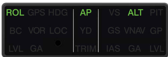
GI 285 AFCS Annunciator Panel Annunciating Alt Hold Mode
