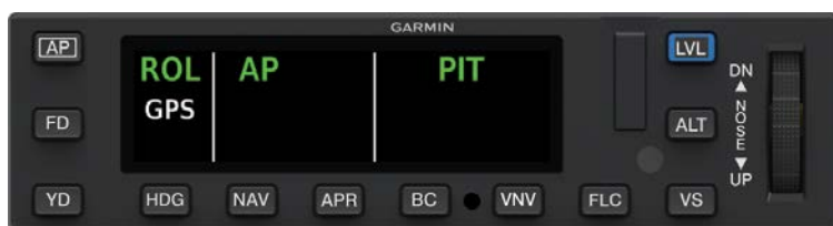
GMC 605C-FLC AFCS Mode Controller with Color Display Annunciating GPS Navigation Mode Armed
