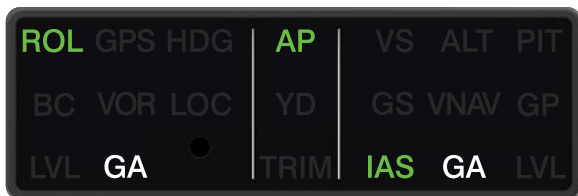
GI 285 AFCS Annunciator Panel Underspeed Indication (Altitude Critical Mode)
