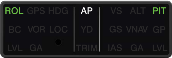
GI 285 AFCS Annunciator Panel Annunciating Control Wheel Steering
