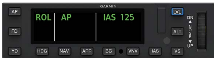
GMC 605C-IAS AFCS Mode Controller with Color Display Annunciating Indicated Airspeed Mode
