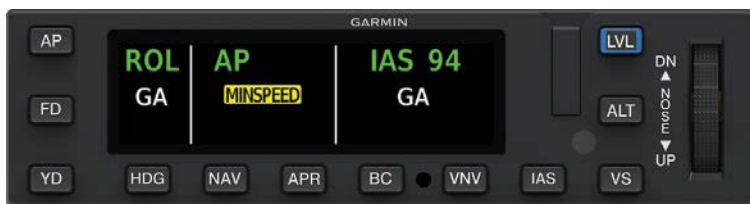
GMC 605C-IAS AFCS Mode Controller with Color Display Underspeed Indication (Altitude Critical Mode)
