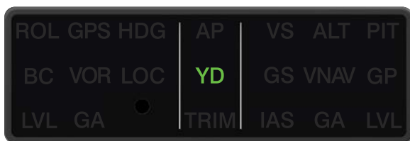
GI 285 AFCS Annunciator Panel Yaw Damper Indication
