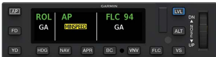
GMC 605C-FLC AFCS Mode Controller with Color Display Underspeed Indication (Altitude Critical Mode)
