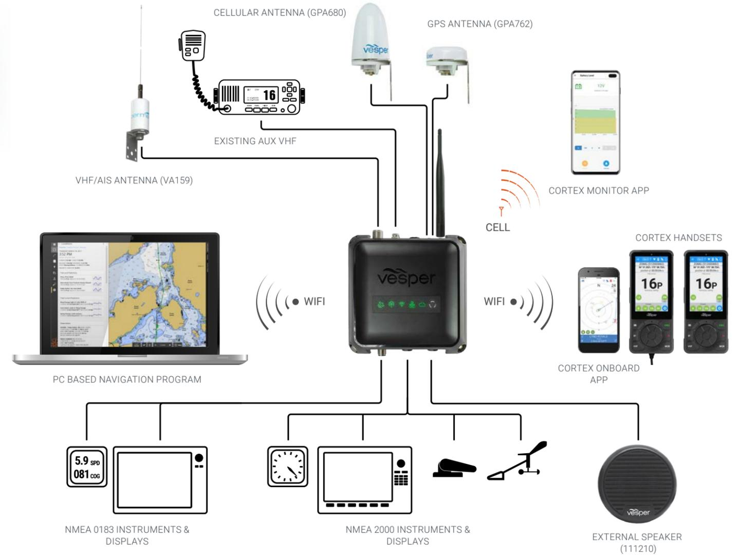
**+** CONNECT TO AN EXISTING ON BOARD NETWORK FOR UP TO 5 ADDITIONAL HANDSETS OR MOBILE DEVICES AND TO ACCESS MONITORING VIA SATELLITE COMMUNICATIONS
