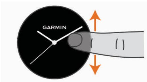
The device scrolls through the widget loop.
