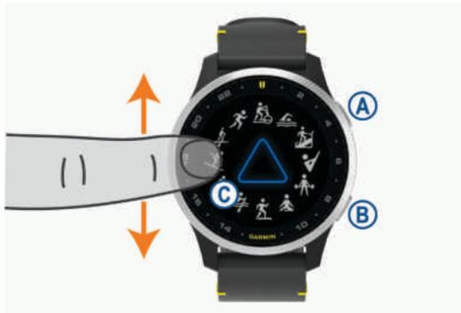
**A Action button:** Press to turn on the device.
