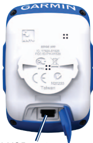
Mini-USB port under weather cap
