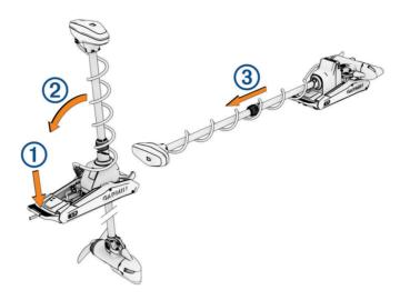
**NOTE:** The motor should automatically steer to 90° for stowing. The propeller stow side can be configured in the settings menu.
