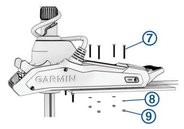
10 Tighten the nuts to a torque of 14.9 N-m (11 lbf-ft.).
