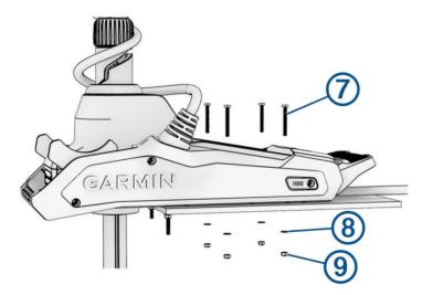
10 Tighten the nuts to a torque of 10.85 N-m (8 lbf-ft.).
