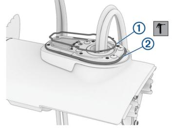
2 Using the grease packet included in the kit, apply grease to the new blue and black motor gaskets included in the kit and install them in place of the gaskets you removed.
