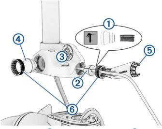
4 Using the included grommet nut wrench (5), tighten the grommet nuts (6).
