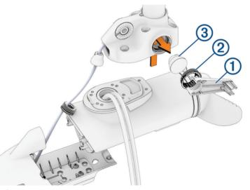
2 Push out the grommets ③ from the inside of the downshaft adapter.
