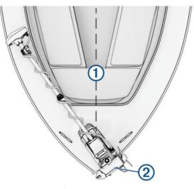
• You must install the mount with the u shape 2 overhanging the gunwale of the boat.
