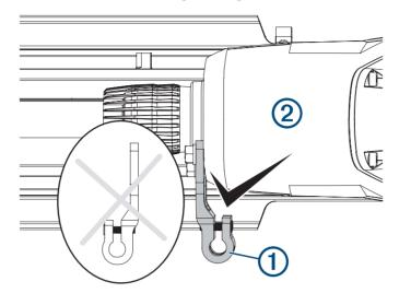
**NOTE:** If you install the bracket with the folded portion facing away from the steering system housing, the stabilizer rod will contact the gunwale and prevent the motor from locking in the deployed position.
