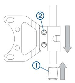
**NOTE:** Two caps are included with the stabilizer. The notched cap fits over the top of the rod and allows you to store the pull handle when it is not in use. You should install the notched cap on the top after you have trimmed the rod in a later step.
