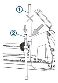
2 Place one of the included upper caps ② on top of the rod to complete the installation.
