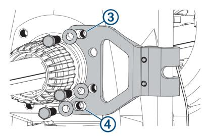
**NOTE:** If you secure the bracket without first pushing it up to rotate it, you may be unable to install the stabilizer rod in the appropriate angle for it to contact the surface under the motor and to allow for the proper clearance when stowing the motor.
