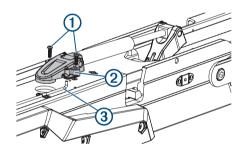
2 Lift the upper gas spring clevis off of the safety rod 3.
