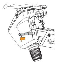
The steering servo is no longer connected to the mount.
