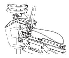
2 Insert the pull cable ① through the bottom half of the handle ②.
