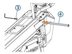
**TIP:** It is helpful to use the other 4 mm hex wrench to hold one end of the upper pin stationary while you remove the screw.
