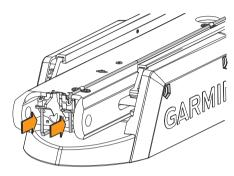
6 Holding the pull cable 4 up, place the steering servo housing onto the lower link of the mount, aligning the lower holes on the housing with the holes on the link.
