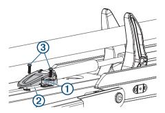
**NOTE:** If you must rotate the gas spring so the base aligns with the mount, rotate the spring in a clockwise direction only. Rotating the gas spring in a counter-clockwise direction may loosen the fittings.
