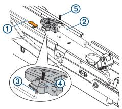
2 If necessary, pivot the upper gas spring ② toward the lower link of the mount so the base of the gas spring aligns with the safety rod and mounting holes.
