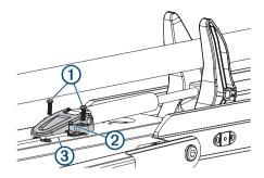
3 Lift the lower gas spring clevis off of the safety rod 3.
