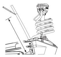
2 If you do not see a mark on the cable, or if the mark is not approximately 40 cm (16 in.) from the connection, make a mark with a marker or tape. 3 With the motor in the deployed position, route the transducer cable through the channel along the right (starboard) side of the mount (1).
