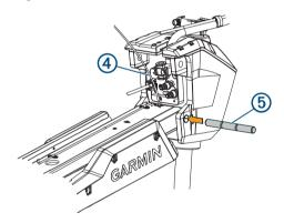
7 While lifting up on the steering servo housing, push the pivot pin (5) through the housing and the link to hold it in place
