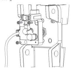
**NOTE:** You may have to lift up on the upper link as much as allowed by the power cable to access the screws that secure the cable-junction box.
