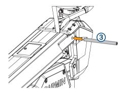
**5** Using a 4 mm hex bit or hex wrench, secure the pin using the screws and washers ④ on both sides.
