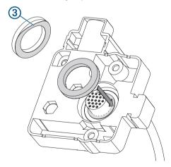
**4** Remove the liner from the adhesive backing **4** on the thin round seal from the kit, position it around the connector on the cable junction box, **adhesive-side down**, and press downward until it is firmly in place.
