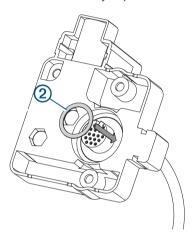
3 Remove the liner from the adhesive backing ③ on the thick round seal from the kit, position it around the connector on the cable-junction box, adhesive-side down, and press downward until it is firmly in place.
