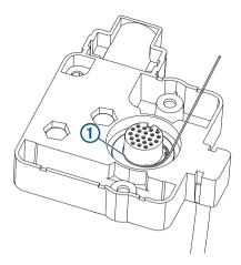
2 Position the small round flat seal (without adhesive) from the kit ② around the connector on the cable-junction box, and press downward until it is firmly in place.
