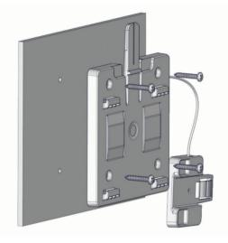
**NOTE:** You must install the bracket with the release tab pointing up to properly secure the amplifier in the bracket.
