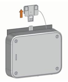
2 Press the tab (1) on the mounting bracket, and lift up (2) on the amplifier to disconnect it from the mount (3).
