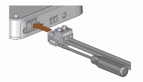
**6** Using a 5 mm  $(^{7}/_{32}$  in.) flat (slotted) screwdriver, secure the power terminal block to the amplifier.
