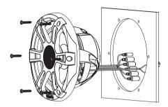
15 Secure the subwoofer to the mounting surface using the included screws.
