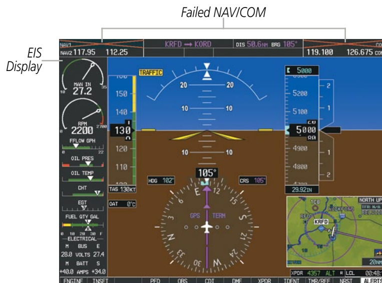
Figure 3-2 Primary Flight Display (182T Reversionary Mode)
