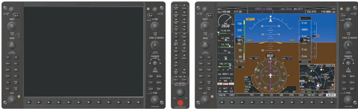
Figure 1-9 Reversionary Mode (Failed PFD)
