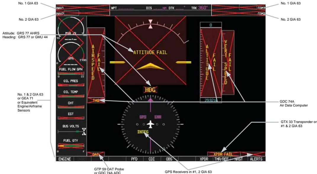
**Figure 3-1. PFD Power-up System Annunciations**
