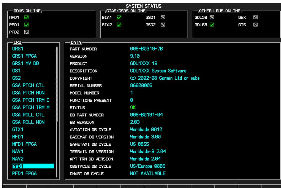
1. Go to the System Status page using the FMS knob. Activate the cursor and toggle to the LRU window.
