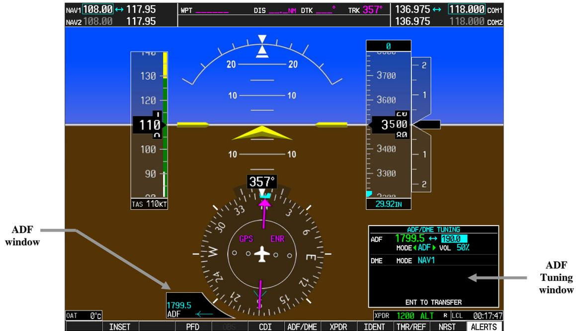
1. On the PFD, check to see if the ADF window(s) is displayed. If not, press the PFD softkey. Using either the BRG1 or BRG2 softkeys, toggle the softkey until the ADF bearing is shown. Press the BACK softkey.
