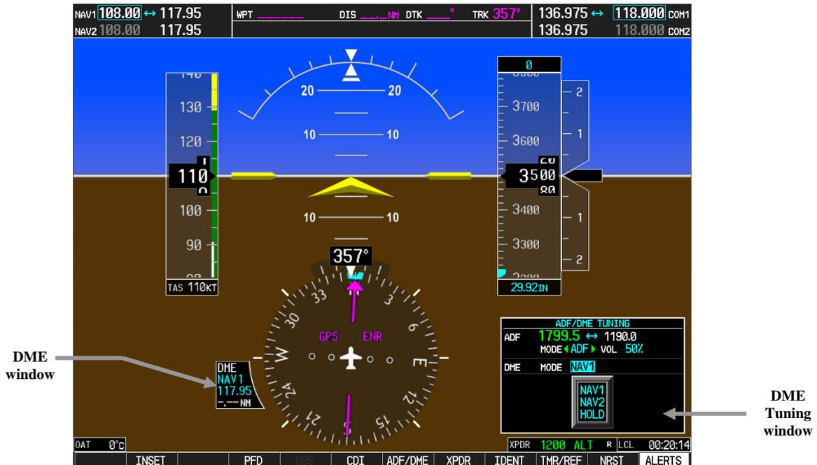
1. On the PFD, check to see if the DME window is displayed. If not, press the PFD softkey, then press the DME softkey to display the DME window next to the HSI.
