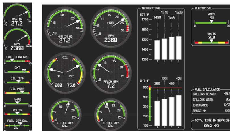
3. Press the RED reversionary mode button on the GMA 1347 audio panel. Verify that engine gauges are display on the MFD and PFD.
