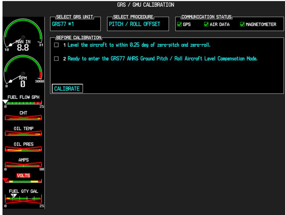
This procedure must be carried out with the engine off. Go to the GRS page group on the PFD. Select the GRS/GMU Calibration page on the PFD.
