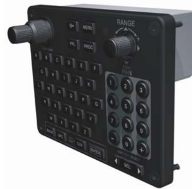
Figure 3-16. GCU 475 MFD Control Unit
