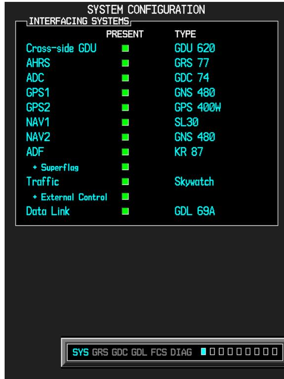
Activate the cursor, select the system using the large MFD knob, and then press the ENT button. This will activate or deactivate the highlighted system. For activated systems, use the small knob to select the appropriate LRU from the dropdown TYPE menu, and then press enter to select the LRU.
