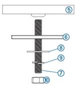
9 Using a torque wrench, tighten the nuts to 13.7 to 18.6 N-m (10 to 14 lbf-ft.).
