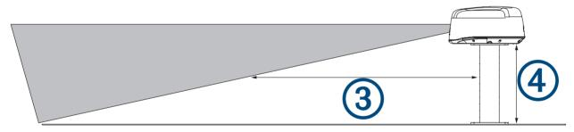
For example, if the mounting location is 2 m (6.6 ft.) from the corner of the roof, this is how you would complete the equation to determine the mounting height after converting to mm (or in.):
