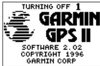
*To prevent accidental battery power loss, the GPS II will automatically shut off 10 minutes after the last keystroke if the unit is not tracking at least one satellite and has never acquired a position fix.*
