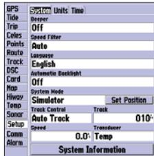
The Set Position, Track Control, Track and Speed fields only show while in simulator mode.
