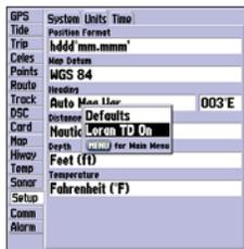
On the Units Tab of the Main Menu, press **MENU**, then highlight 'Loran TD On' and press **ENTER** to select Loran TD.
