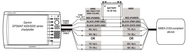
Wiring to a Standard NMEA 0183-compliant Device for One-Way Communication
