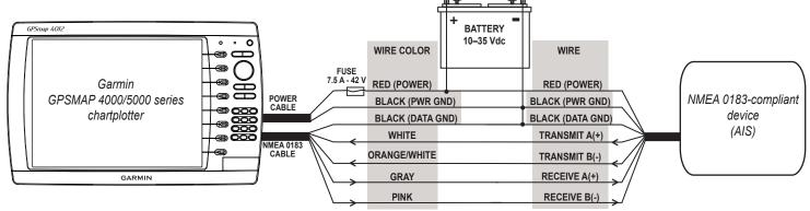
Wiring to a NMEA 0183-compliant Device (AIS)
