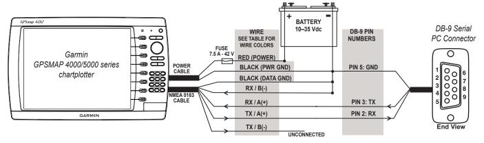
Wiring to a DB-9 Serial PC Connector
