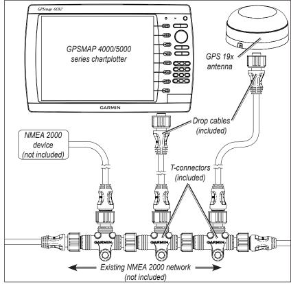
Connecting the GPSMAP 4000/5000 Series Chartplotter and GPS 19x
