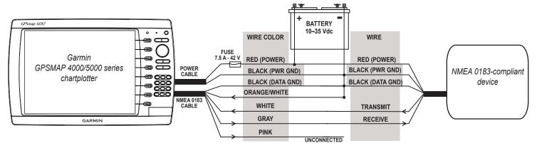
Wiring to a Single-ended NMEA 0183-compliant Device
