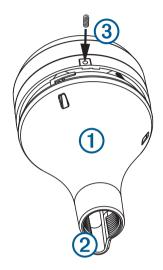
2 Screw the pole-mount adapter onto a standard 1 in. OD, 14 threads per inch, pipe-threaded pole (not included).
