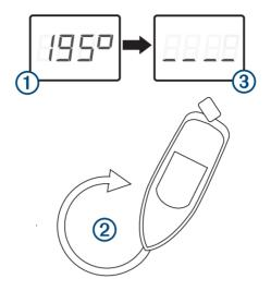
6 Within three minutes, complete two full, slow, tight circles 2, taking care to keep the boat as steady and level as possible.
