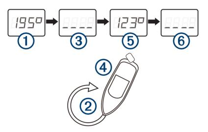
6 Within three minutes, complete two full, slow, tight circles ②, taking care to keep the boat as steady and level as possible.
