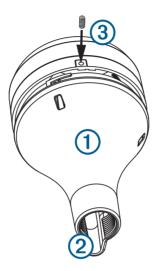
2 Screw the pole-mount adapter onto a standard 1 in. OD, 14 threads per inch, pipe-threaded pole (not included).
