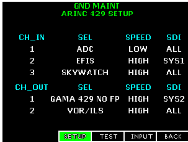
Figure 2-13 GNS 480 ARINC 429 Setup
