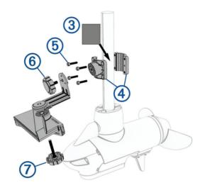
**NOTE:** The rubber liner is not needed when installing the transducer on a trolling motor with a shaft diameter larger than 25 mm (1 in.).
