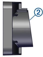
**NOTE:** The trolling motor shaft bracket has an 8-degree angle to reduce the effects of the trolling motor barrel interference with the transducer beam.
