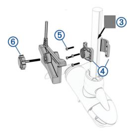
**NOTE:** The rubber liner is not needed when installing the transducer on a trolling motor with a shaft diameter larger than 25 mm (1 in.).
